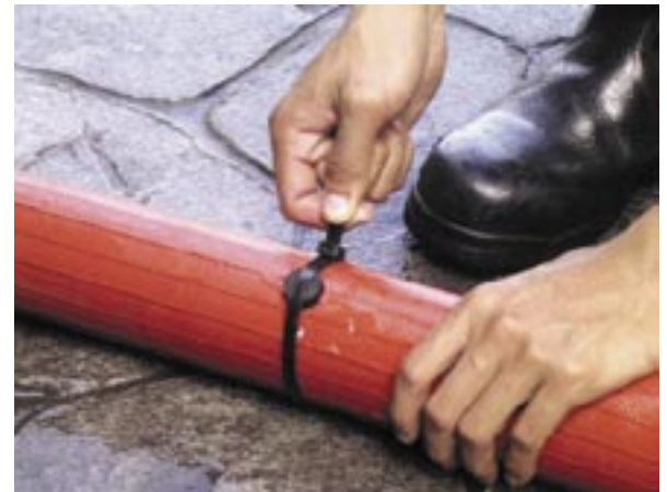
Tightening the cable tie helps to hold the HELP firmly against the leaking hose and relieve the water pressure exerting on the leak spots.
