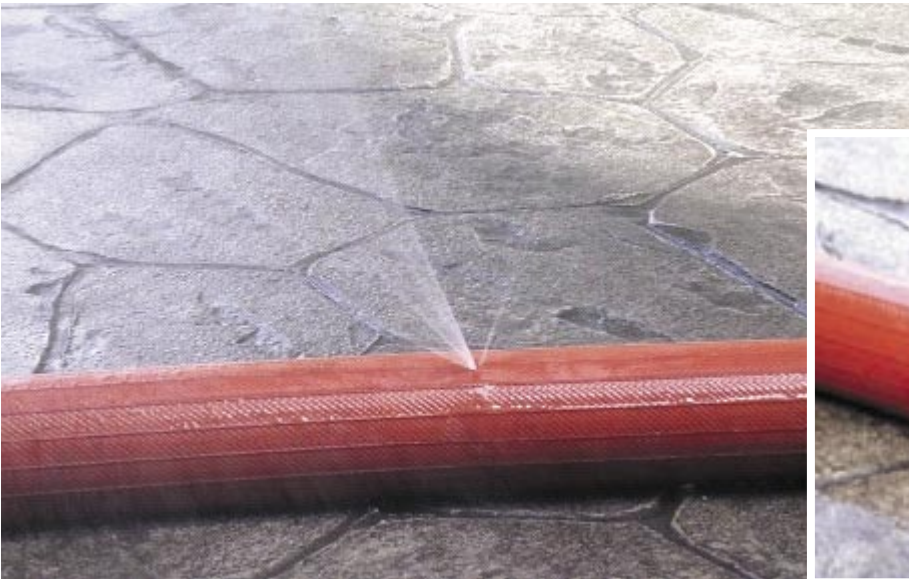
Constant friction between uneven road surfaces and fire hoses often leads to pin-hole leaks in fire hoses as shown above.
