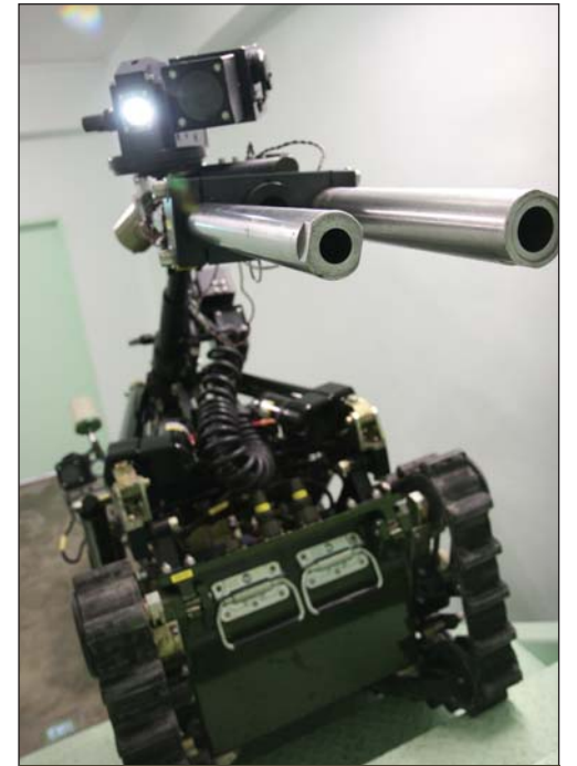
The Wheelbarrow Mark VIII robot can navigate obstacles and staircases to locate and neutralise CBRE threats. It can be remotely controlled to provide visual feedback on a situation, or destroy an IED.
