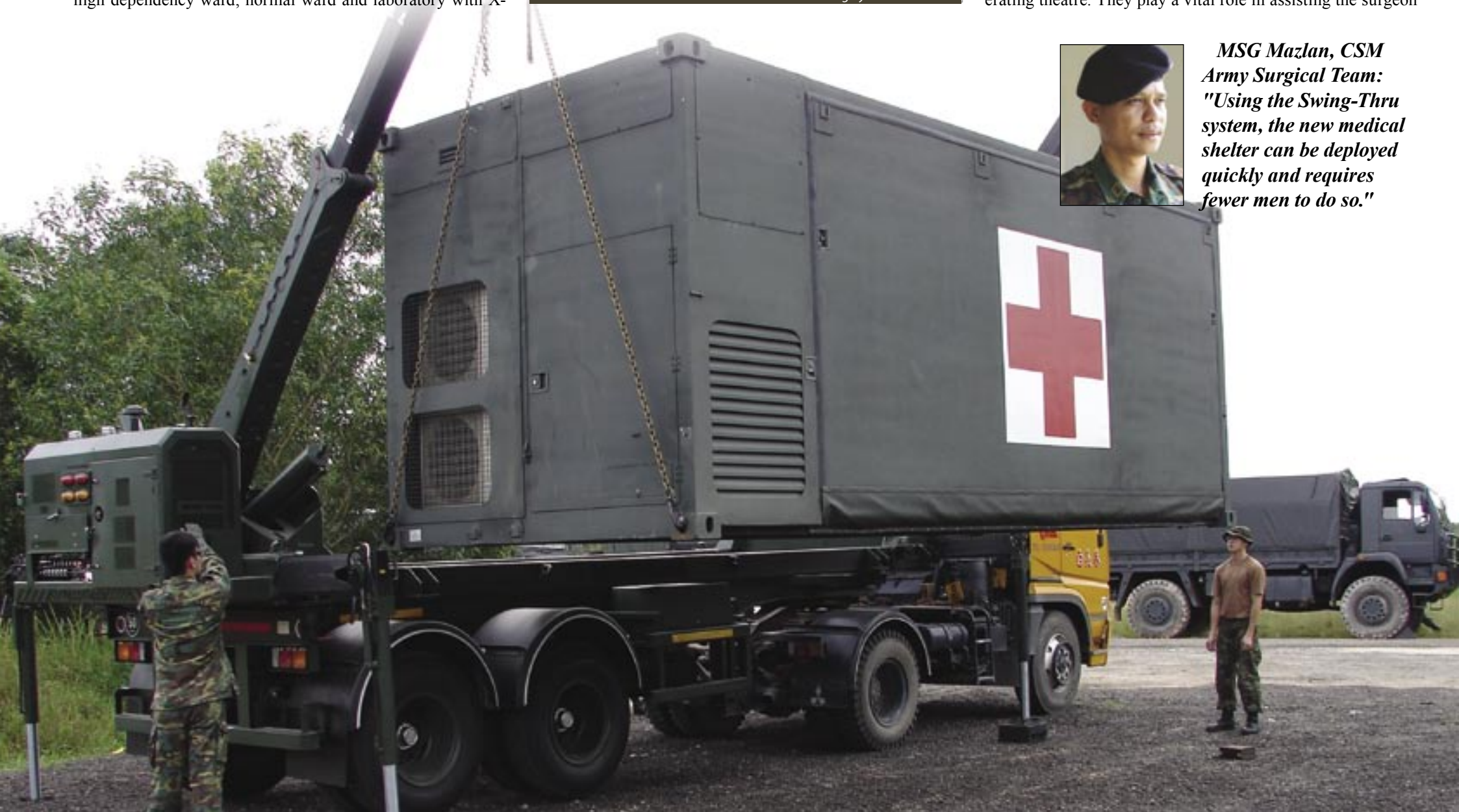
The Rapid Deployable Medical Shelter offers an air-conditioned environment for sterile surgery
