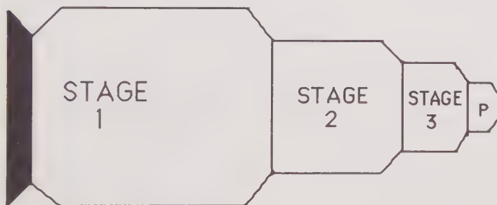
Schematic of the rocket staging principle.
