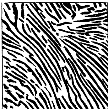
Fig. 20 Structure of pearlite \times 1000 approx.
