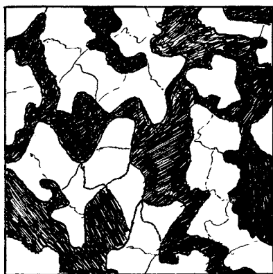
(a) Normal structure of ferrite and pearlite
