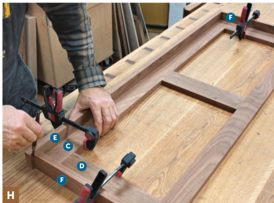
To mark the length of the frame rails (E), clamp the frame stretchers (F) flush with the edge of a seat support rail (C). Align an end of a frame rail with the outside face of a frame stretcher and mark the rail.
