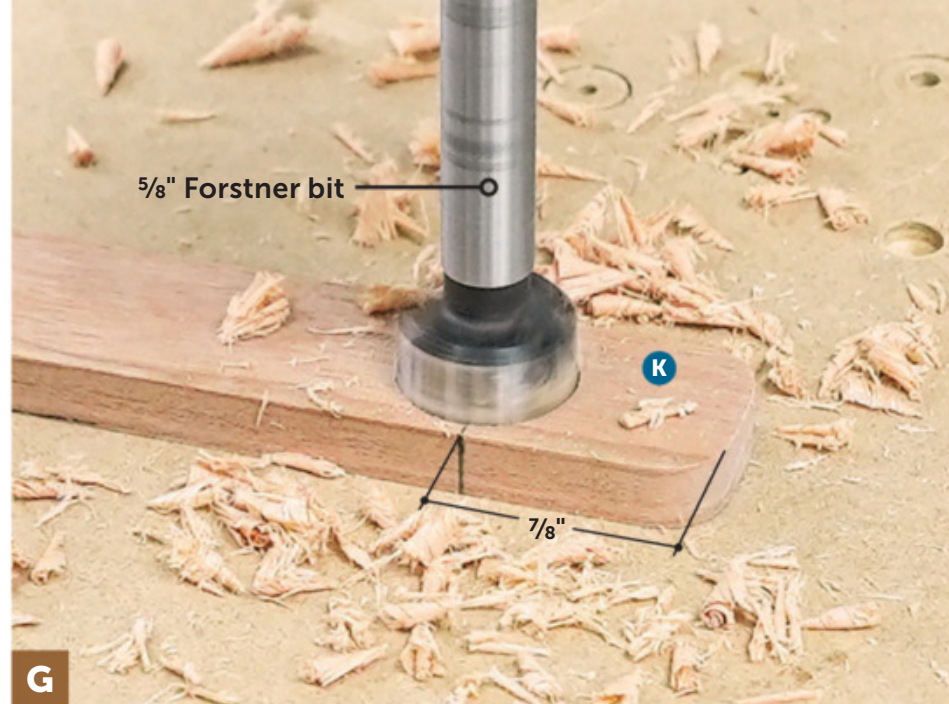
G To form the hitch shroud (K), round the corners on the end of a long blank, then drill a hole centered on the width. Crosscut the part to finished length at the midpoint of the hole.
