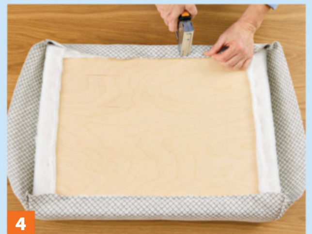
4 Roll enough of the unfinished edge of the fabric under to allow stapling through it. Work from the center to one corner, pulling the fabric taut as you go. Then repeat toward the other corner.
