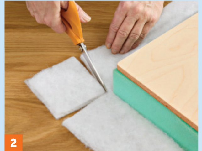
2 Align the scissors with the edge of the foam and cut away each corner of the batting layers. This reduces bulk at the corners, making it easier to fit the fabric covering.
