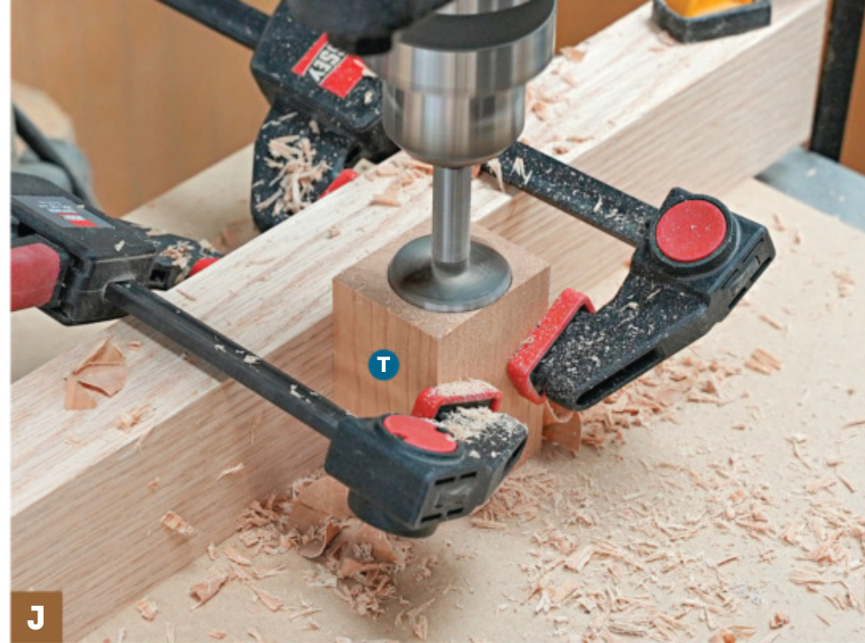
Clamp the boiler jacket (T) to a vertical support to bore the large hole in the end grain. Then drill holes in the top for the sand and steam domes (W, X).
