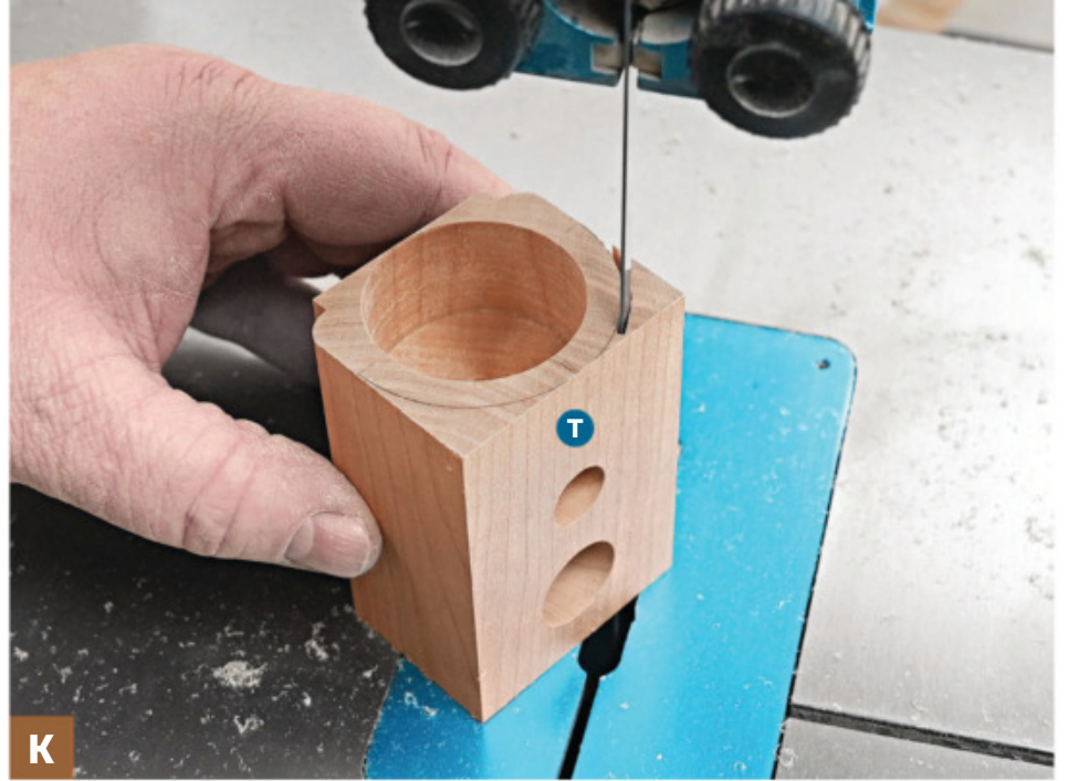
K Cut the radius on top of the boiler jacket (T) by standing the piece on end at the bandsaw. Cut just outside the layout line, then sand the curve smooth.
