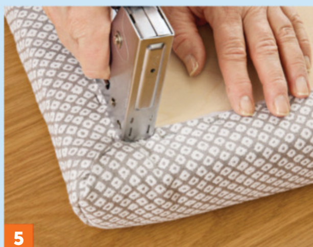
5 After stapling along all four edges, reload your stapler with \frac{5}{16} " fasteners. Gather up the loose fabric at a corner into a triangle. Fold the triangle over, keeping it taut, and secure it with several staples.
