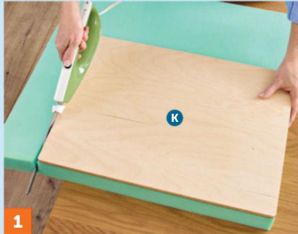
1 Use an electric knife or a serrated bread knife to trim the foam. Keep the blade against the plywood seat pan (K) and perpendicular to its face.
