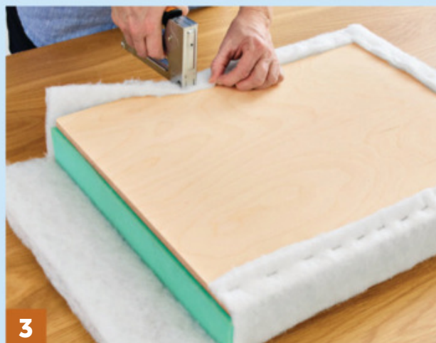
3 Fold the batting up on a long edge, aligning its notched end with the edge of the foam and seat pan. Staple along the length, then repeat as you work your way around.
