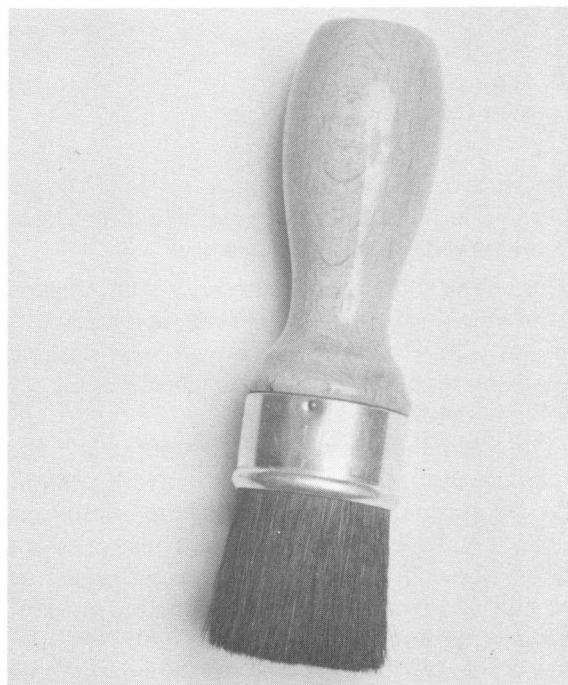
FIG. 163 Ordinary stencil brush can be cut to shape for inking.
