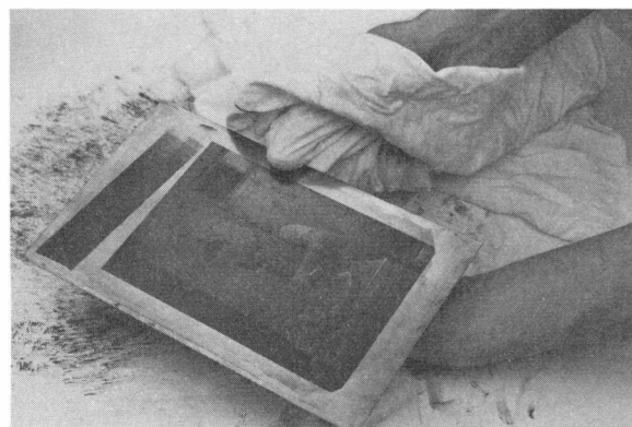
FIG. 218 Wipe the edges of the plate before printing.
