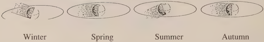
Figure 20. Geosynchronous orbit eclipse, once per orbit, spring and autumn only (TRW)
