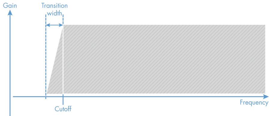
Figure 5-42: The transition width of a filter
