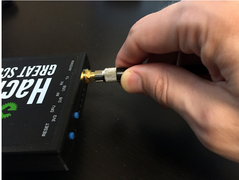
Figure 9-6: Attaching the ANT500 to the HackRF
