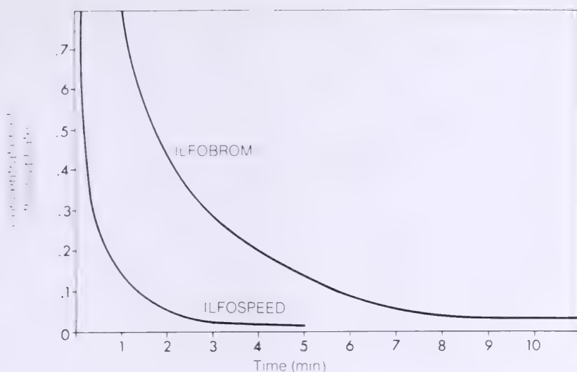
Rate of removal of thiosulfate from resin-coated and fiber-based papers
