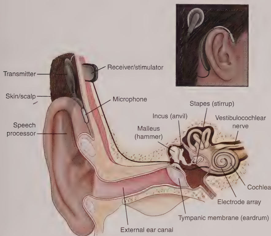
FIGURE 48.3 Cochlear implant. The cochlear implant does not restore normal hearing but does give profoundly hearing-impaired patients representation of sounds to facilitate their understanding of speech.
