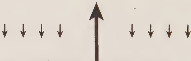
Figure 3.6. Sketch illustrating a strong updraft, represented by the large arrow, and surrounding weak downdrafts, represented by the small arrows.
