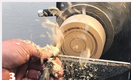
2 A waste block is turned and recesses formed for casting the ring and central disk.
