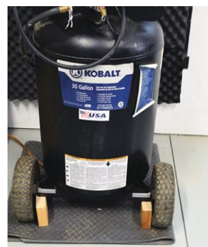
A mat under the air compressor diminishes sound transmission to the floor.
