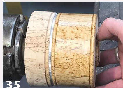
Fine-tune the fit of the lid. The author decides to add a bead on the lid to mirror the one just under the pewter ring.
