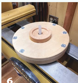
The back of the author's off-center vacuum faceplate. Note the vacuum hose.
