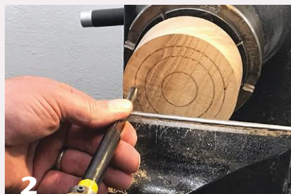
2 A waste block is turned and recesses formed for casting the ring and central disk.
