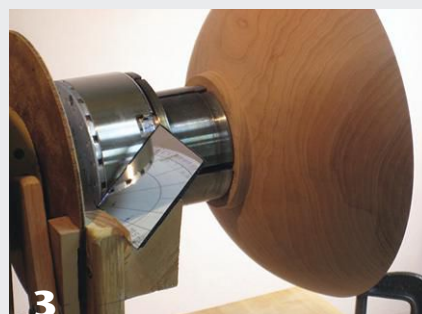
3 An angled mirror allows for sighting across the top of the vertical piece without having to bend down to the centerline of the spindle for each division line.
