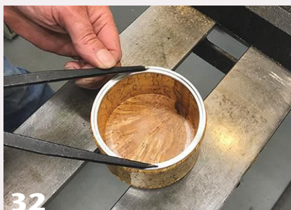
Use dividers to transfer the target diameter to the lid blank.
