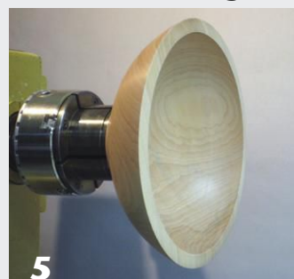
5 The bowl turned and sanded, ready for indexing.
