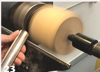
The author uses a spindle-roughing gouge to turn the box to a cylinder.
