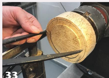
Use dividers to transfer the target diameter to the lid blank.
