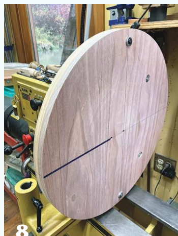
A 20" off-center faceplate with adjustable counterweights on the back.
