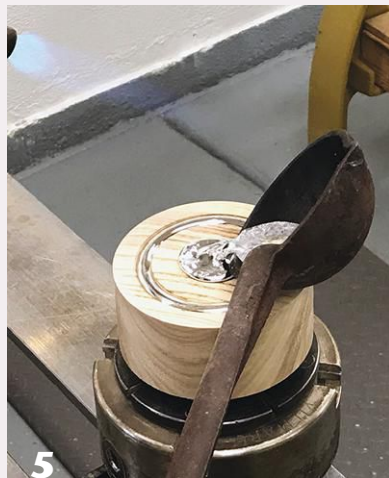
5 Melt the pewter with a torch, then pour it into the mold.
