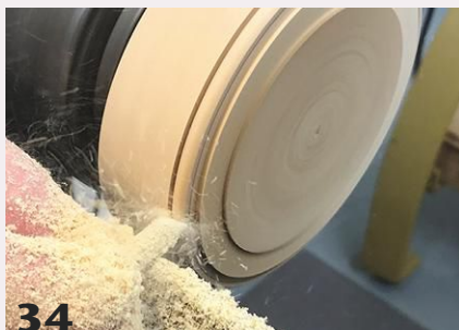
Fine-tune the fit of the lid. The author decides to add a bead on the lid to mirror the one just under the pewter ring.
