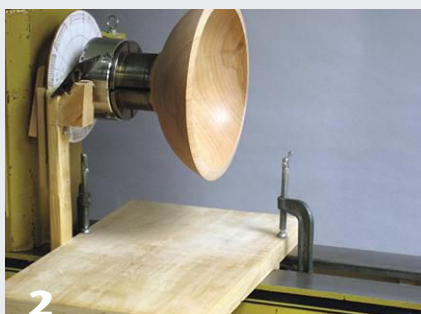
2 Mount the disk, or polar grid, with the paper facing the tailstock. The author uses a chuck to hold the disk in place, but a faceplate up to 6" in diameter could also be used. The plywood base is clamped to the bed ways.
