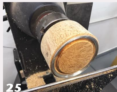
Sneak up on a good fit of the pewter ring to the box rim.
