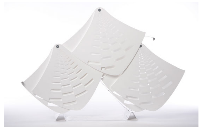
Overlapping shifting elements employing a shape-memory coil spring actuator to produce a translation movement – shown here in the open state (left) and the closed state. The demonstrator is known as “Chameleon Membrane”.
