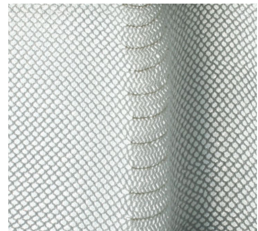
Varying transparency of a 3D textile by bending and compressing the deck layer
