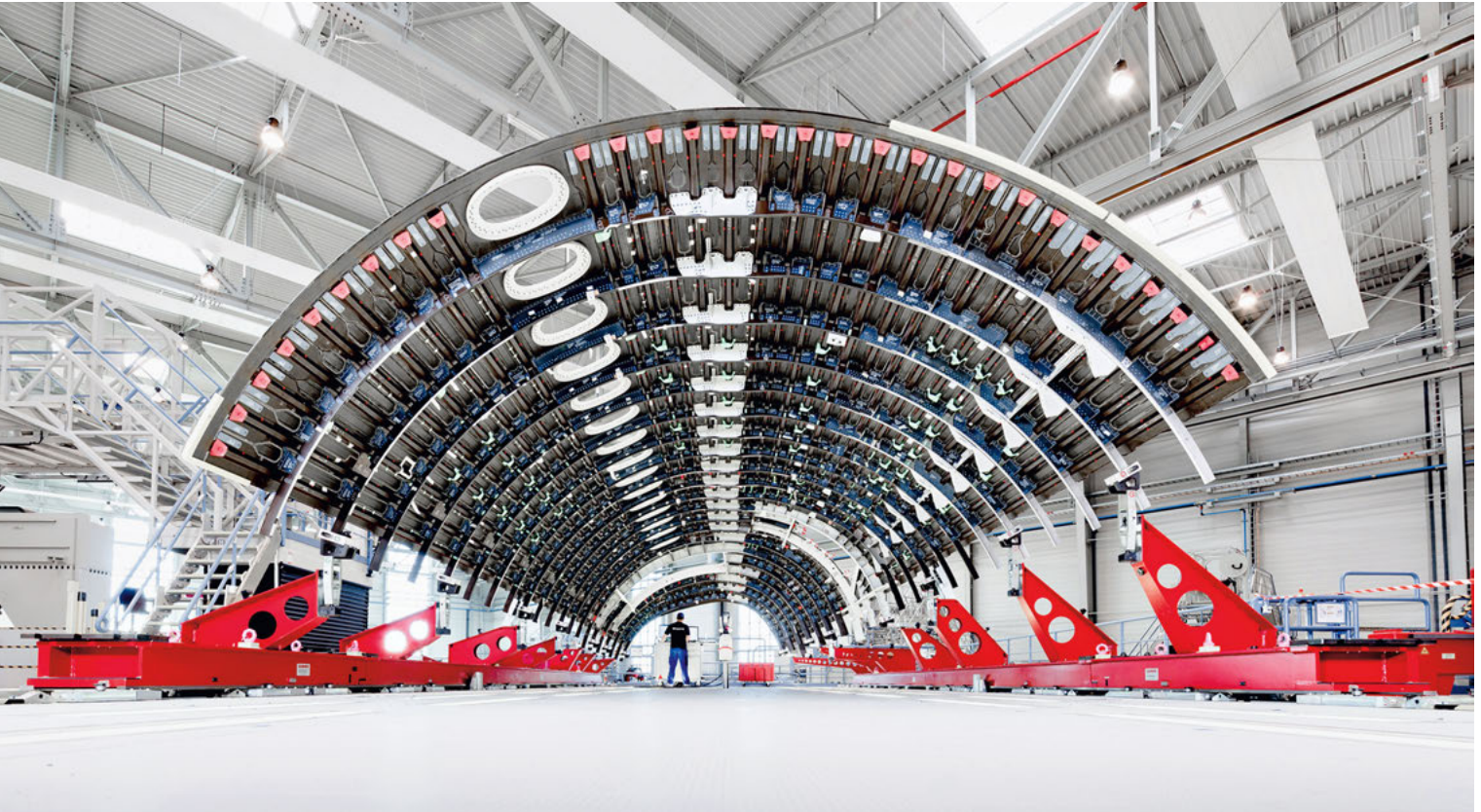
CFRP fuselage shell of an Airbus A350
