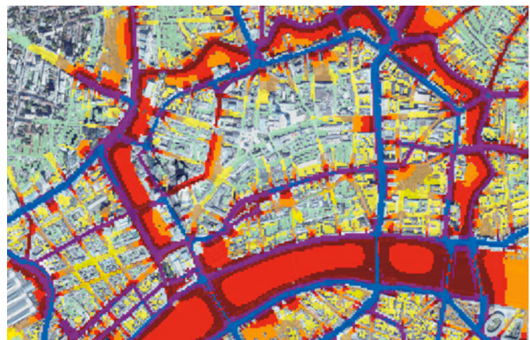
Noise map for the centre of Frankfurt am Main with the main railway station on the right
