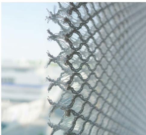
Varying transparency of a 3D textile by shifting the deck layers parallel to each other
