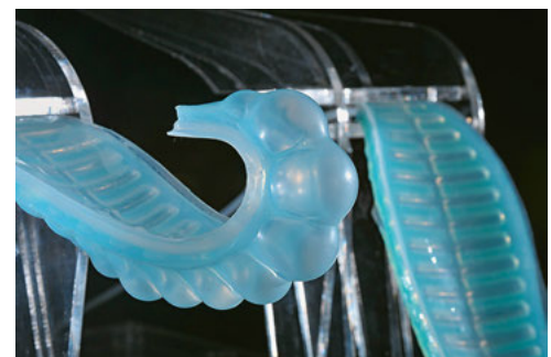
Concept for a pavilion using cast silicon actuators. Using pneumatic actuators, endless patterns and movements can be produced in the pavilion's enclosure.
