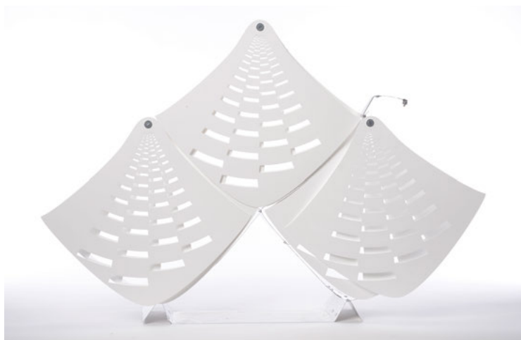
Overlapping shifting elements employing a shape-memory coil spring actuator to produce a translation movement – shown here in the open state (left) and the closed state. The demonstrator is known as “Chameleon Membrane”.
