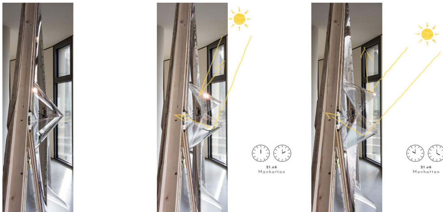
Model of the Dancing Facade: a single system that incorporates deflection of the sun's rays as well as glare and solar protection
