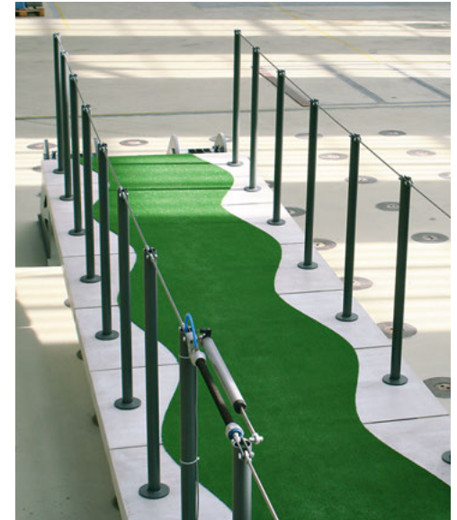
Pneumatic muscle actuator (black) with displacement sensors to measure the degree of deformation
