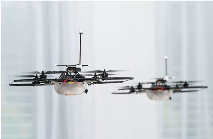
Airborne pixels made using a combination of drones, coloured LEDs and a light control
