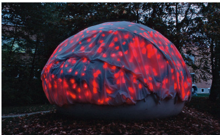
“Paul” – an experimental structure with a multifunctional textile skin on the ILEK site
