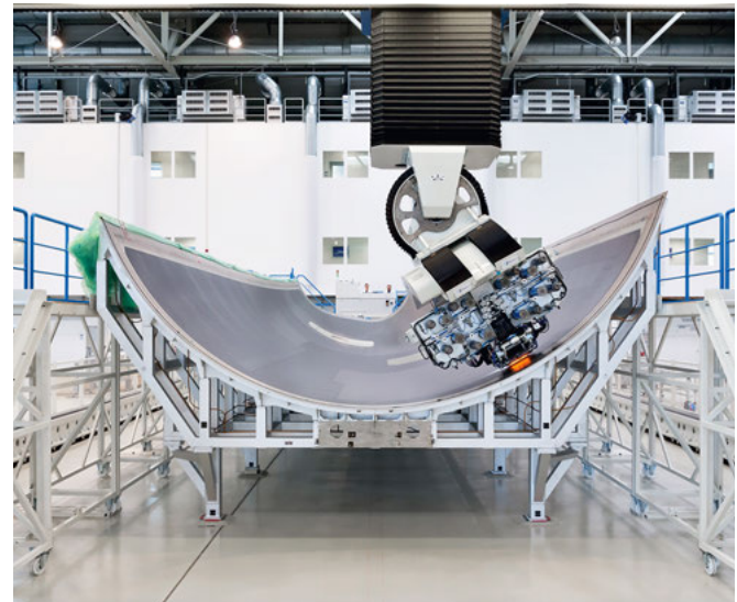
Automated manufacture of an A350 side panel by Premium Aerotec using Automated Fibre Placement
