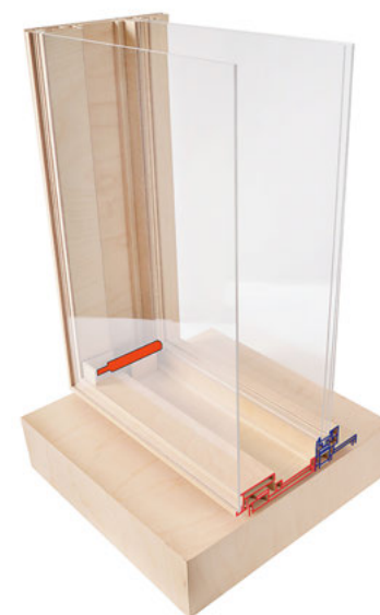
Model of a double-skin facade with an autoreactive actuator
