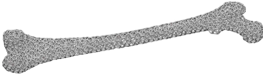
Figure 10.1 This femur model, generated from an SDF, is specifically made to be porous. Porosity is important so that implants can grow properly into living tissue.
