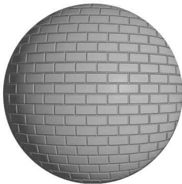
Figure 9.12 Normal mapping affects the normal vectors only in the shading computation. It doesn't add any "real" geometry to the scene.
