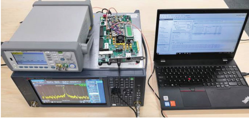
Fig. 6.47 The experimental platform for evaluating AOBS SSCG
