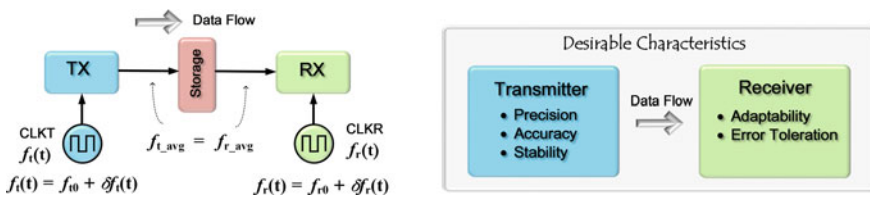
Fig. 5.8 Flexible clocking strategy for the basic operation of data transfer
