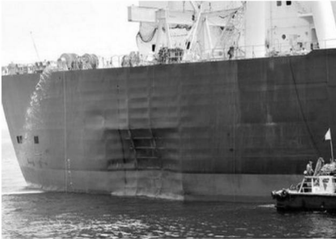
Damage to the hull of the M. Star. (Emirati News Agency photo.)
