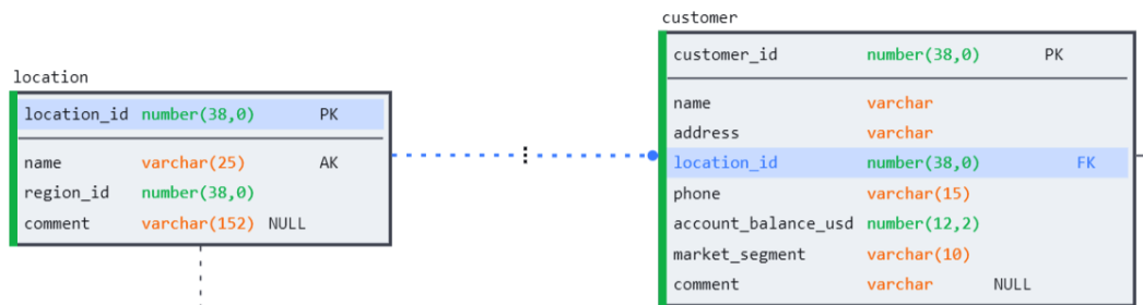
Figure 12.1 – Foreign key constraint between location and customer tables
