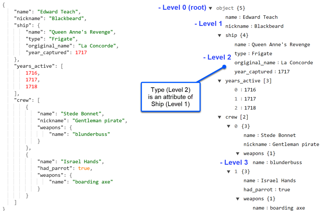
Figure 15.5 – Observing the number of nested levels in a semi-structured object
