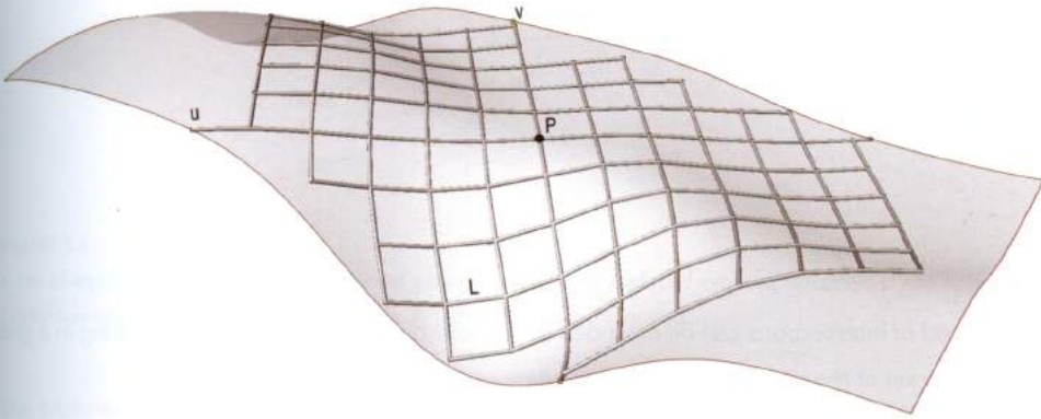
FIGURE 3.8 A grid of equal-length edges generated on an arbitrary freeform surface.
