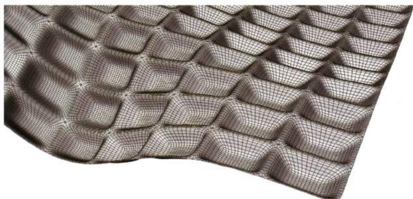
FIGURE 6.14 The final mesh resulting from the subdivision operated by the Catmull-Clark component.
