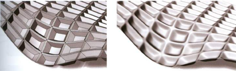
FIGURE 6.13 Smoothing a tridimensional skin by a subdivision strategy based on the Catmull-Clark algorithm.
