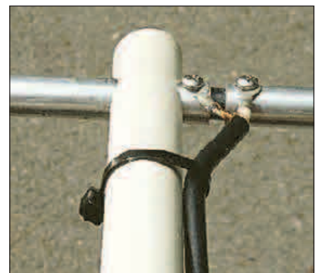
Figure 8 — A close-up of the junction of the support arm, the dipole element, and the connecting cable termination for portable operation. For a permanent installation, insert a stainless steel washer between the hook connector and the element and seal the junction.
