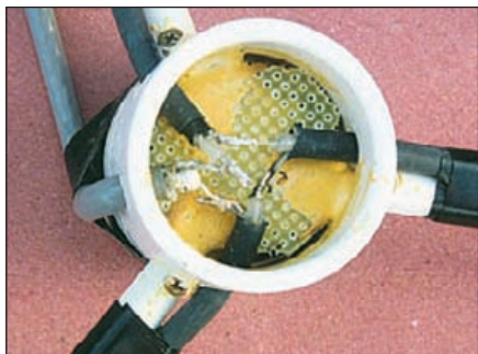
Figure 10 — The hub, support rods and the main junction of connecting cables and the 1/4 matching section before final sealing.
