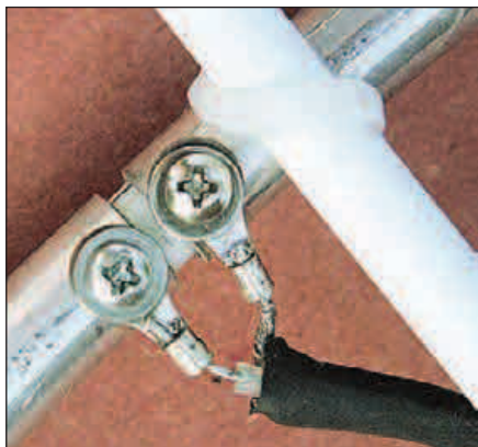
Figure 9 — A close-up of the method used to connect the element to the support arm with cable ties in the circular antenna.
