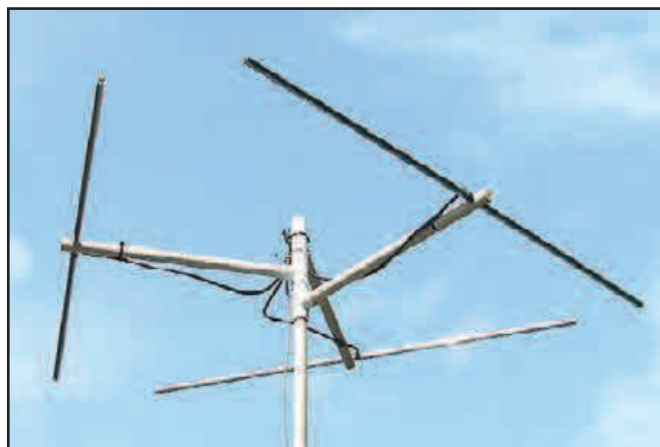
Figure 7 — An overall view of the HPOD triangle in use, showing the general construction and cable routing.
