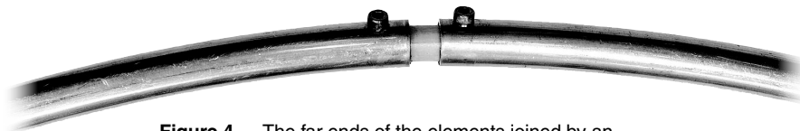
Figure 4 — The far ends of the elements joined by an insulating fiberglass rod. The gap is precisely \frac{5}{16} inches long.
