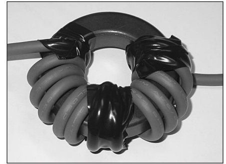
Figure 5.50 — A ferrite choke consisting of multiple turns of cable wound on a 2.4-in. OD × 1.4-in. ID × 0.5-in. toroid core.
