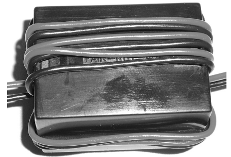
Figure 21.73 — RF choke for screwdriver antenna control and power leads.
