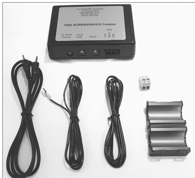
Figure 21.76 — A screwdriver antenna controller made to work with the IC-7000 transceiver.
