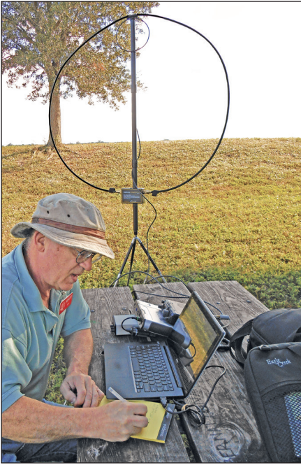
Figure 21.59 — A typical small loop being used for portable operation with a QRP transceiver. Be sure to account for minimum safe distances to avoid excessive RF exposure levels.
