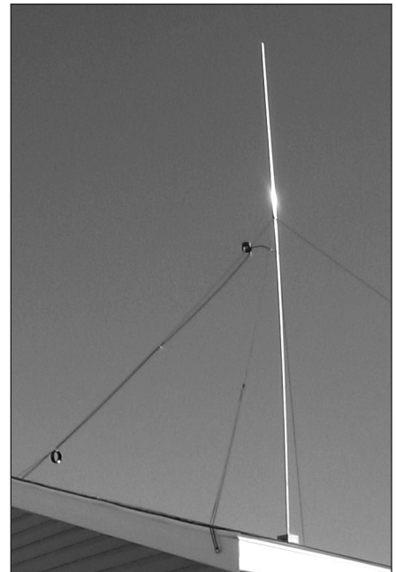
Figure 21.45 — The HVD installed at K8CH. An eye screw that is used for securing one of the guy lines is visible in the foreground. You can also see the two choke baluns that are used in the feed system (see text).
