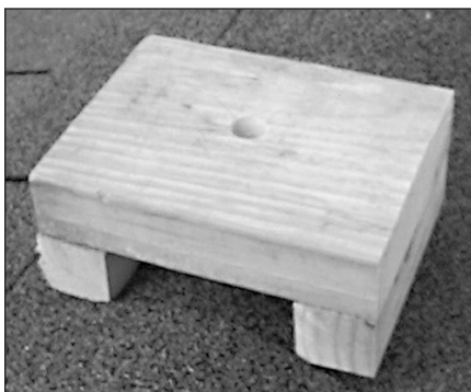
Figure 21.44 — At K8CH, the HVD base insulator sits in this saddle-shaped wooden fixture. This was photo was taken before the fixture was painted — a necessary step to protect against the weather.
