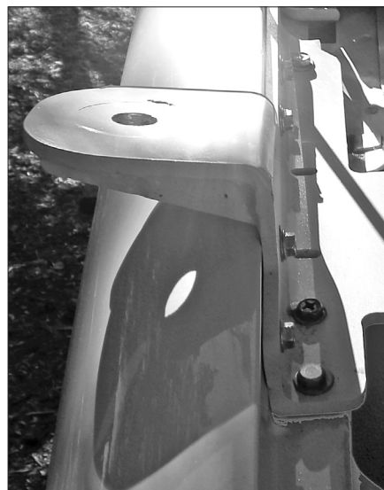
Figure 21.79 — The KE5DKM bracket mounts under the hood of a motor home.
