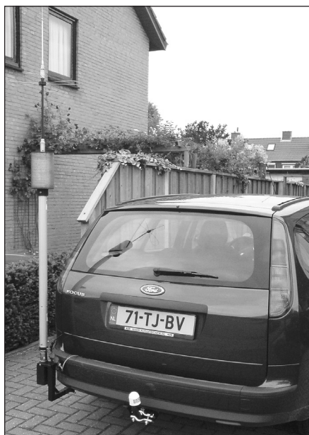
Figure 21.77 — The PA3VOS antenna mount easily supports a large screwdriver antenna and is offset to allow the hatch to open and close without removing the antenna.
