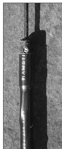
Figure 21.70 — Continuously-loaded whip antennas are short and lightweight. The base section consists of a fiberglass tube wound with wire to form the loading inductor. At the top of the base section the length of a steel whip or stinger can be adjusted to bring the antenna to resonance. [Joel Hallas, W1ZR, photo]
