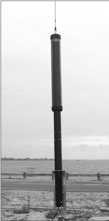
Figure 21.72 — The screwdriver-style remotely-controlled whip antenna. A small motor in the base mast moves a coil past contacts at the top of the metal base section. The top whip section is attached to the top of the coil. As the coil moves out of the mast, more inductance is connected in series between the base section and top section. Screwdriver antennas are popular because they offer multiband coverage. [Joel Hallas, W1ZR, photo]
