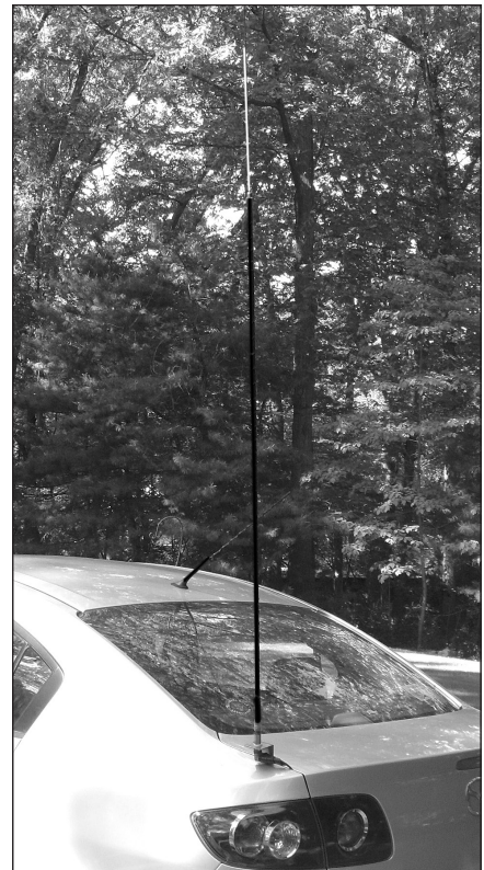
Figure 21.70 — Continuously-loaded whip antennas are short and lightweight. The base section consists of a fiberglass tube wound with wire to form the loading inductor. At the top of the base section the length of a steel whip or stinger can be adjusted to bring the antenna to resonance. [Joel Hallas, W1ZR, photo]
