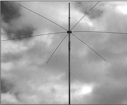
Figure 21.34 — W9SR’s short vertical uses top loading and a capacitance hat with a 10 foot TV mast to make a compact antenna for 160, 80 or 40 meters.
