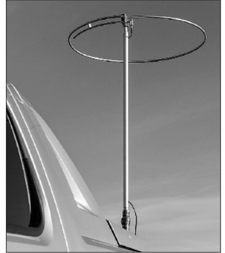
Figure 21.82 — The halo is a popular horizontally polarized mobile antenna for 6 meters through 70 cm. This version was made by Jerry Clement, VE6AB, and the construction article is available online (see text).
