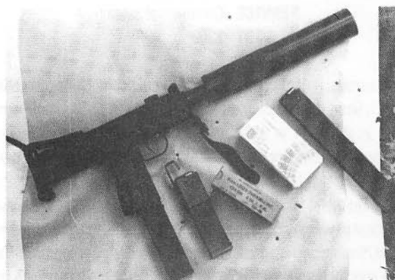
Ingram M11/9mm with Interand suppressor showing both 15 and 30 rd magazines
