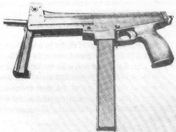
JATI MATIC with front handygrip/safety unfolded
