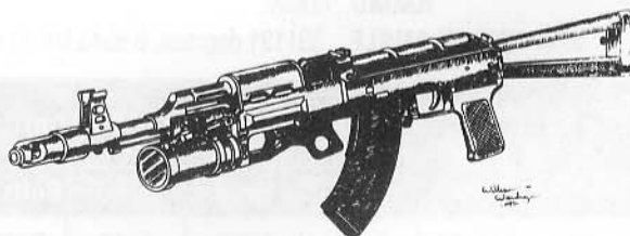
AKS-74 with BG-15 mounted under the front grip
