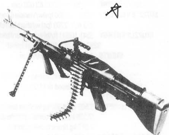
M60E3 with long barrel
