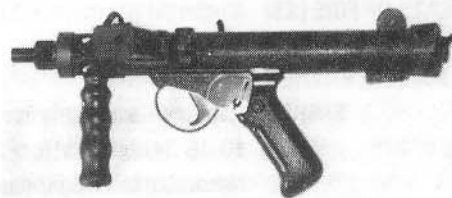
Sterling Mark 7A4 with bolt forward and 15 rd magazine
