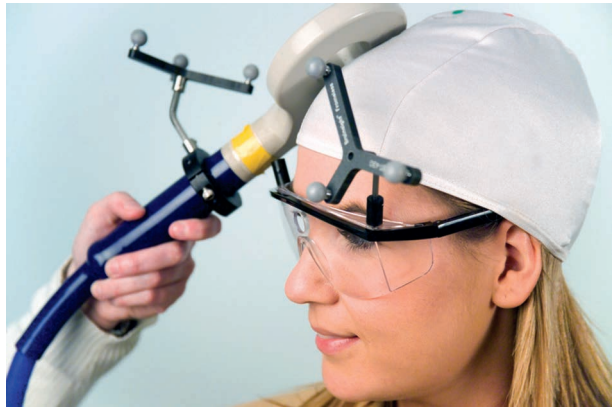
FIGURE 5.13: The coil is held against the participant's head, and a localized magnetic field is generated during performance of the task.
