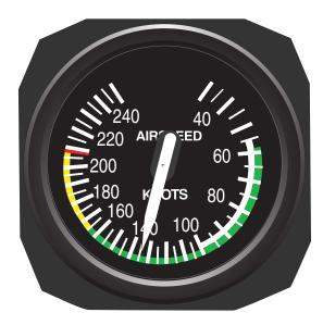
Figure 7-48 Airspeed indicator.
