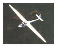
Figure 1-44 High aspect ratio.
