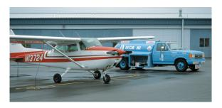
Figure 6-3 Fueling from a tanker.
