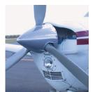
Figure 5-26 Check propeller is clean.
