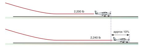
Figure 9-13 A 10% increase in weight requires a 10% increase in landing distance (approximately).
