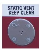
Figure 7-4 Static vent.
