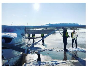
Figure 3-51 Snow, ice, and frost must be removed from all surfaces prior to flight.
