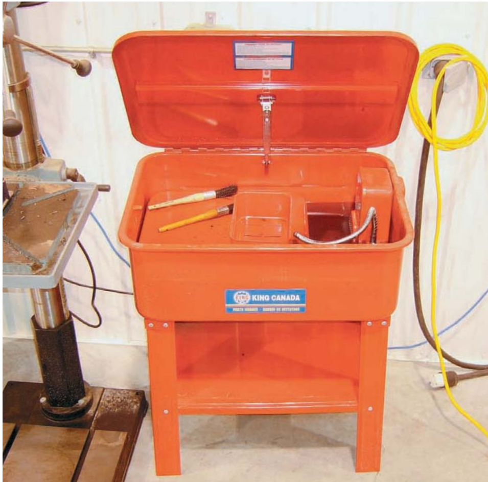
A large floor model solvent parts washer expands the range of parts that can be cleaned.
