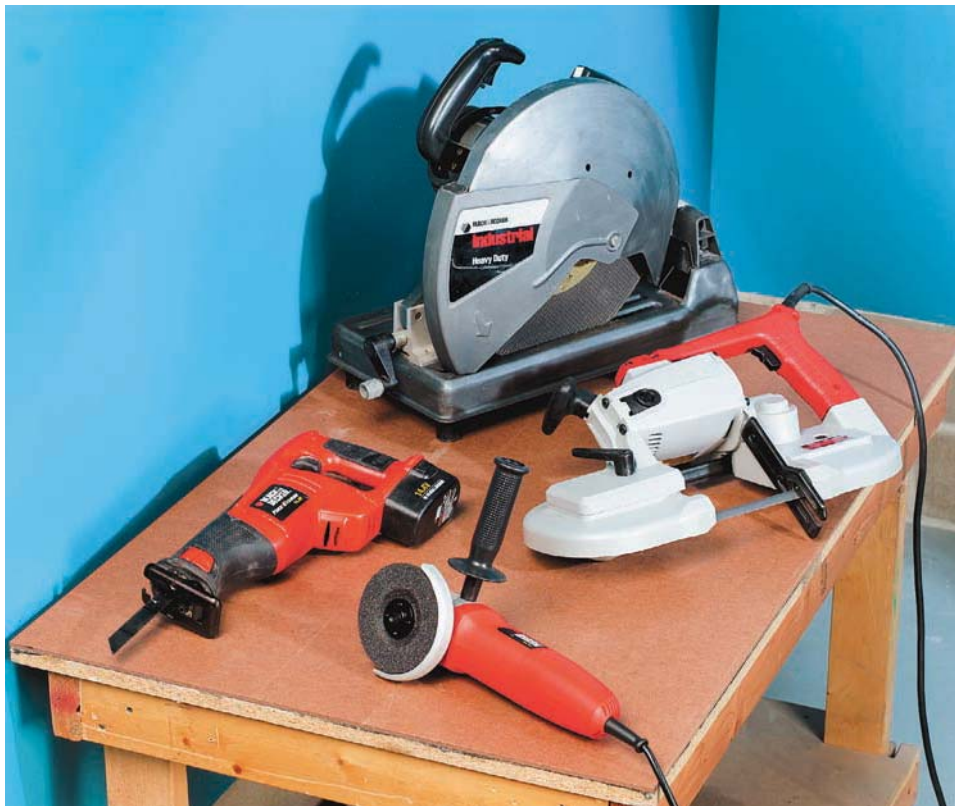
Power tools for a welding shop include: (A) reciprocating saw, (B) cut-off saw, (C) portable band saw, (D) angle grinder.
