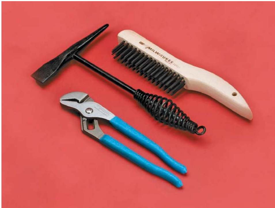
Useful tools for shielded metal arc welding are a pliers, chipping hammer, and wire brush.
