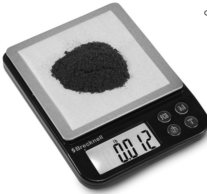
Photo 2.13 Brecknell EPB-3000 pocket scale with readability of 0.1 grams and a capacity of 3000 grams.
