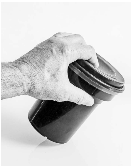
Photo 6.4 At the end of either four inversions or 10 seconds, gently tap the edge of the tank on the sink or counter top to dislodge air bubbles. It is not necessary to tap the tank hard.
