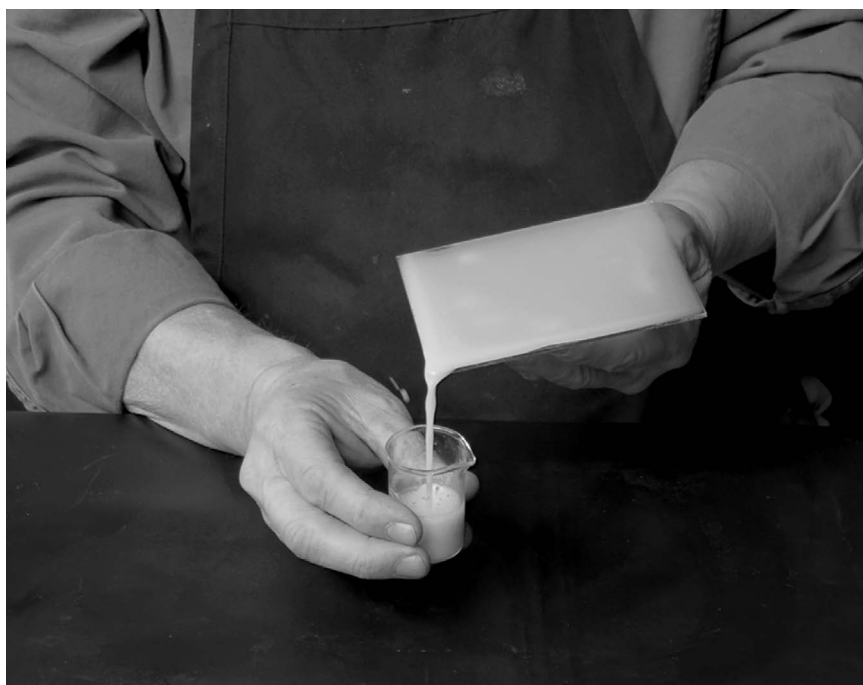
Photo 18.6 Slightly tip the plate to let some of the emulsion flow off one corner and back into the pouring cup.
