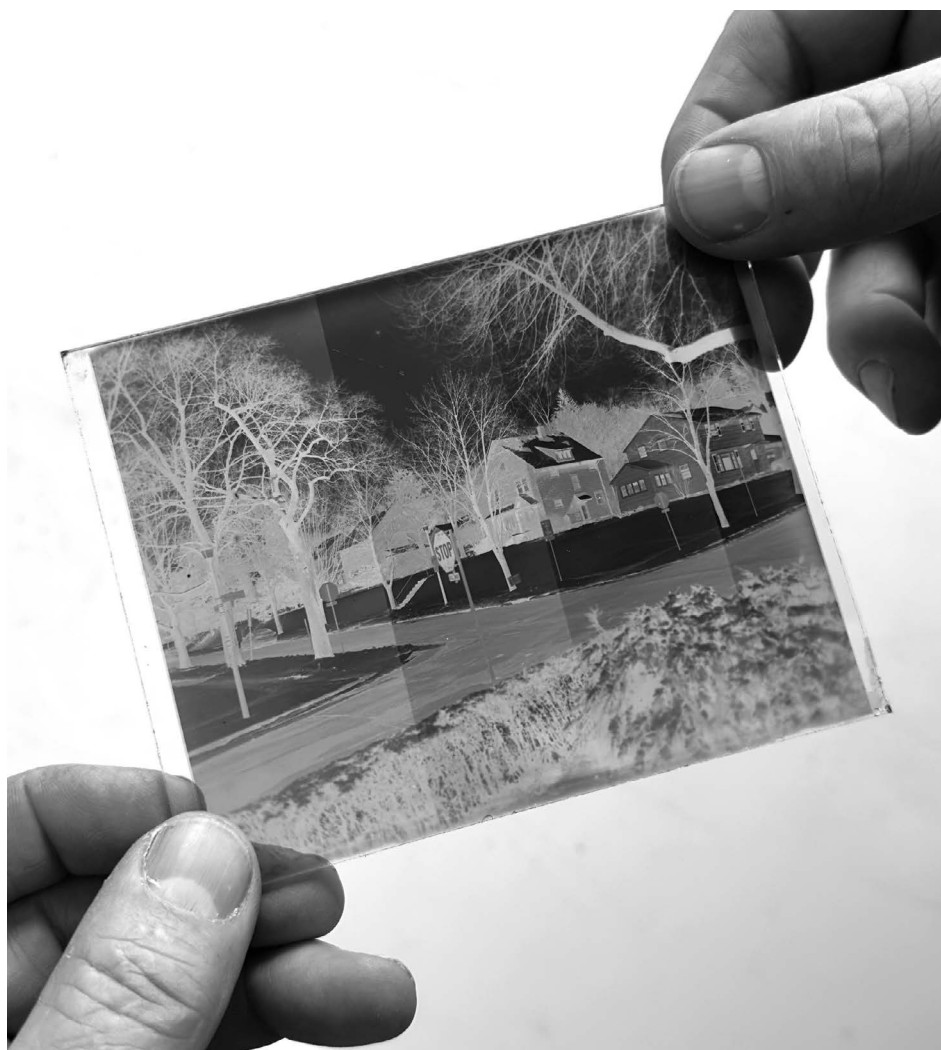
Photo 18.7 An exposure test negative on an MO-1880 gelatin dry plate. Developed by inspection with Dektol.
