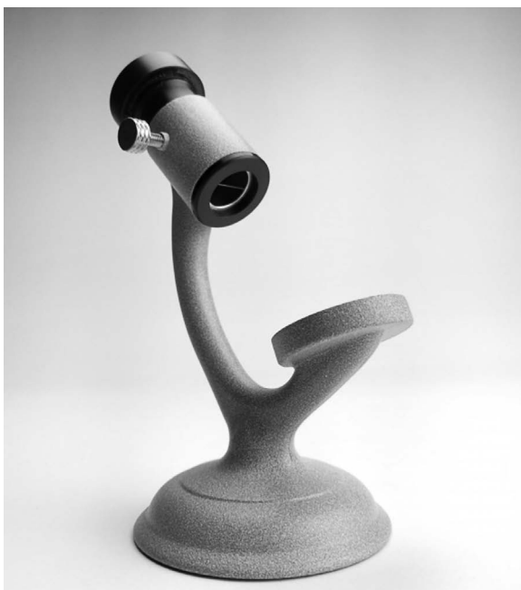
Photo 2.4 Grain focuser. It is only possible to critically focus a negative with a grain focusing device such as this one. Avoid grain focusing devices made of plastic and focus finders that don't specifically say "grain focuser." These focus on the image, not the grain, and while they are better than nothing, they are not as accurate.
