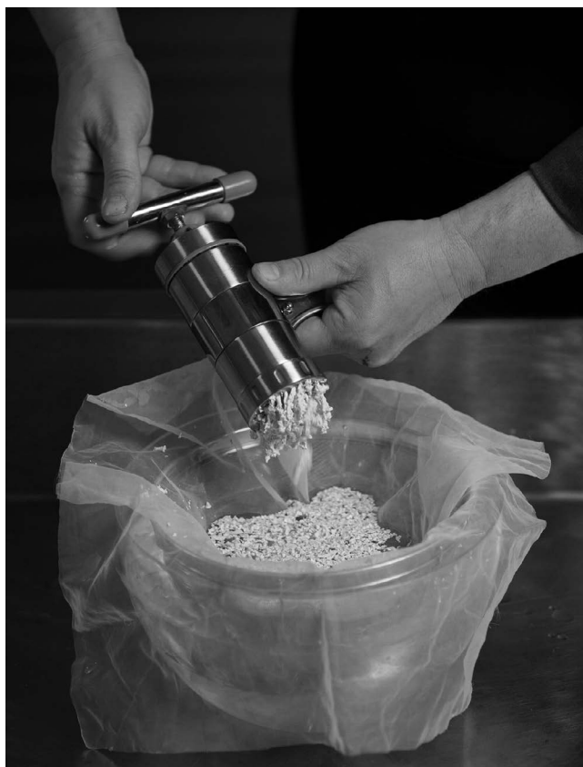
Photo 18.2 Noodling. Squeeze the noodler to extrude emulsion noodles that will fall into the center of the fabric.
