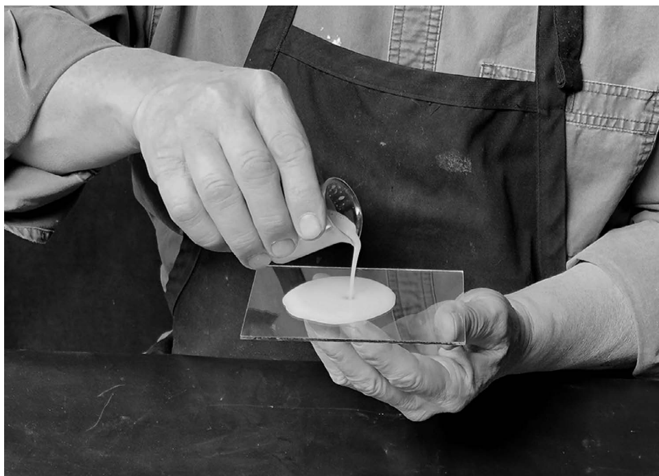
Photo 18.4 Pour the 25 mL emulsion onto the center on the plate.
