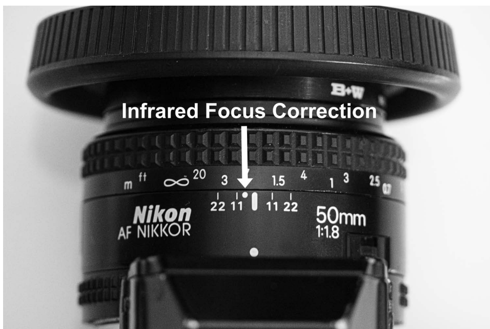
Photo 3.2 IR-Engraving on Lens. If there is an IR focus point engraved on your lens, focus on your subject, then move the focus point to the IR focus point. The focus point is often designated by a dot, as seen on this Nikon lens. Some lenses have a short red vertical dash, or there might be the letter "R." In this image, the lens was focused at 7 feet. The 7-foot mark was shifted to the IR indicator for correct focus.
