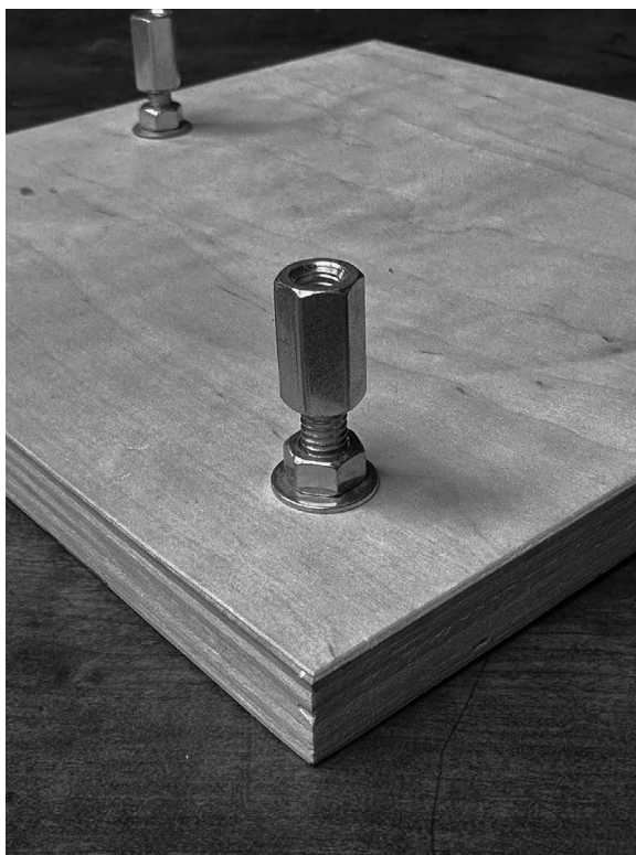
Photo 18.9 Install the bolts and attach the washers and nuts to the bolts on the underside of the plywood.
