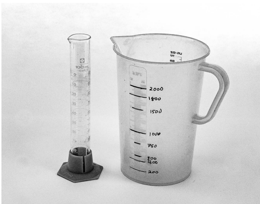
Photo 2.8 Graduate and beakers. A graduate is a tall cylinder for accurately measuring volume. A beaker is a wide vessel for mixing chemicals. If you want volume, use a beaker; if you want accuracy, use a graduate.
