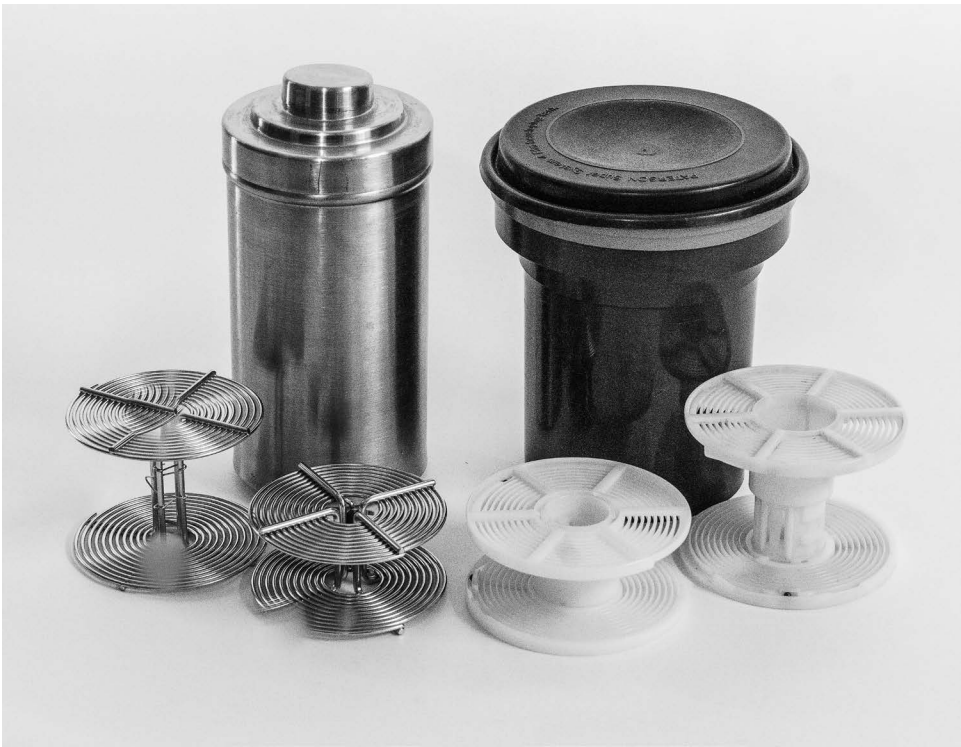
Photo 2.6 Developing tanks. It makes no difference which type of tank you use; use the one you are more comfortable with. It is the volume of developer per 80 2 inches of film and the agitation method that will change the quality of your negatives. I highly recommend at least 300 mL per roll.
