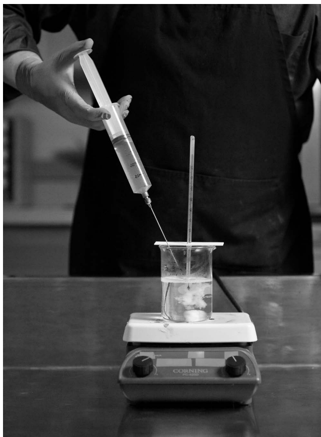
Photo 18.1 Precipitation of the silver solution into the promo-iodized gelatin solution.
