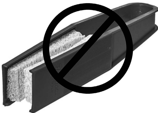
Photo 2.19 Bad film squeegee. A big no-no. How fast can you spell scratched film?
