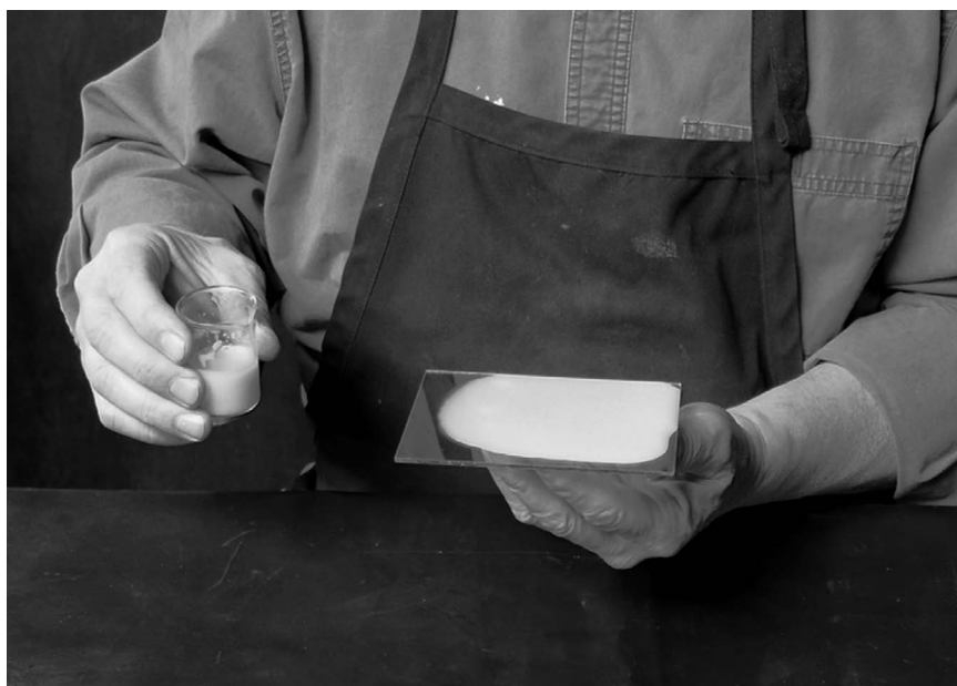
Photo 18.5 Distributing the emulsion across the surface of the plate.
