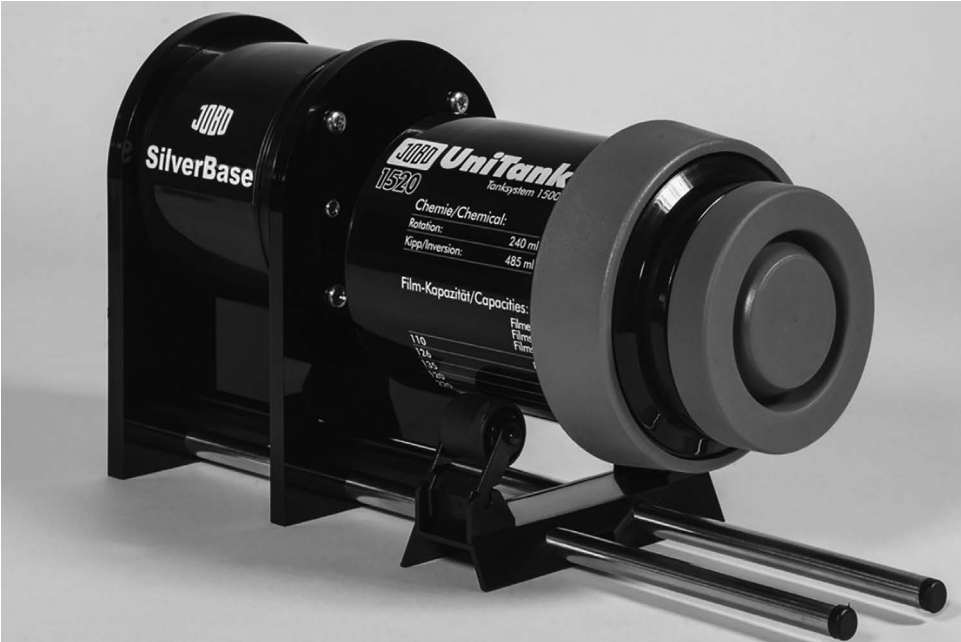
Photo 6.2 If you use continuous agitation, you may wish to invest in a SilverBase Rotary Processor.
