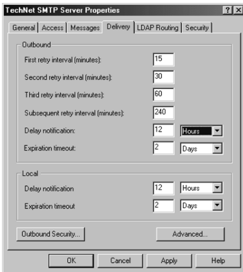
Figure 8-14. Use the options of the Delivery tab to control message delivery in the organization.
