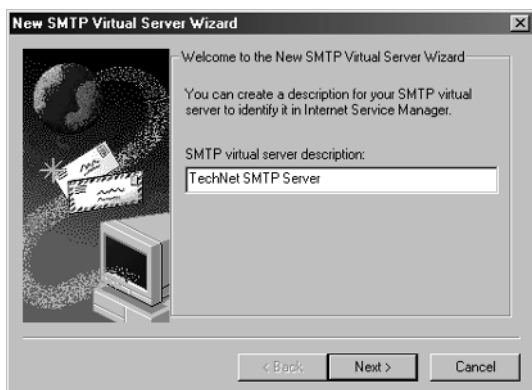
Figure 8-1. Use the New SMTP Virtual Server Wizard to create the additional virtual server.
