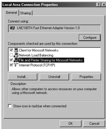
Figure 10-11. Use the Local Area Connection Properties dialog box to configure file and printer sharing settings for the Web server.
