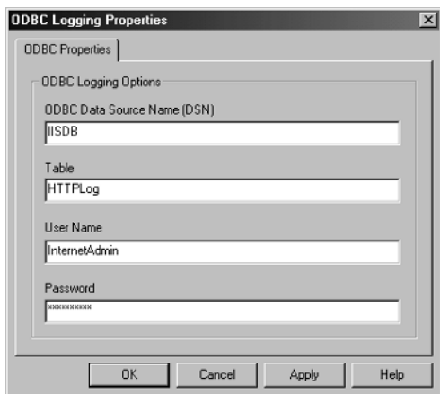
Figure 11-6. Use ODBC logging when you need to write to a database.
