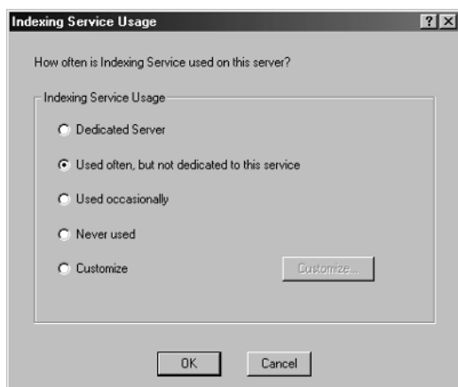
Figure 9-3. Use the Indexing Service Usage dialog box to optimize indexing and querying.
