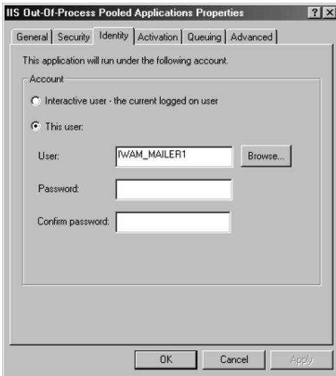
Figure 5-2. Set the Web application account identity in the Component Services snap-in.
