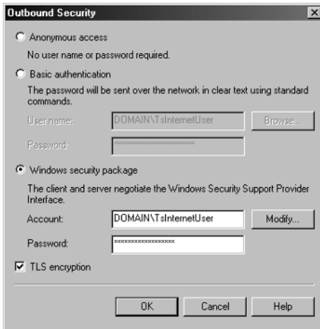
Figure 8-8. Select the outbound security options and add TLS encryption if supported by the remote domain.
