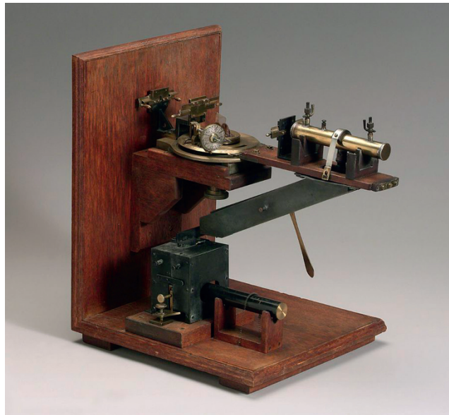
Figure 6.4 X-ray diffractometer (1912) used by the W.H and W.L. Bragg to investigate the crystal structure of minerals. Adapted from https://en.wikipedia.org/wiki/William_Henry_Bragg#/media/File:X-ray_spectrometer,_1912._(9660569929).jpg .
