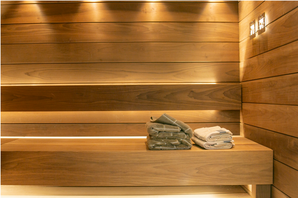
Figure 140. First generation LED and fiber lighting created spotlight effects, the new versions illuminate smooth arcs and planes. The source of light itself can be hidden. This installation uses 3,000 K LEDs.
