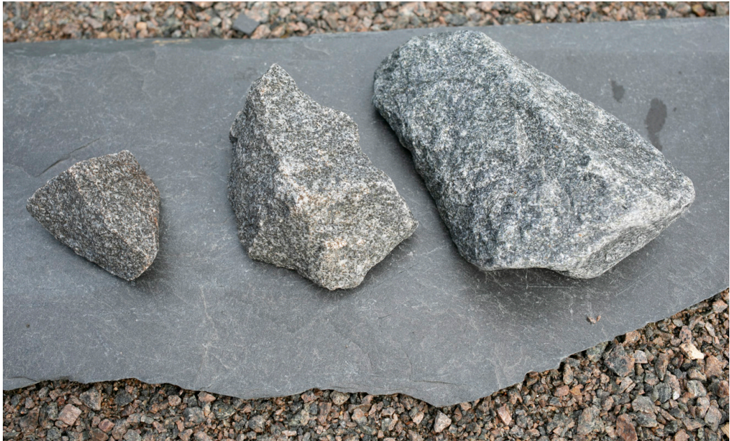
Figure 85. The three sizes of Finnish sauna stones produced from natural stone: small, medium, and large. All samples are made of olivinediabase.
