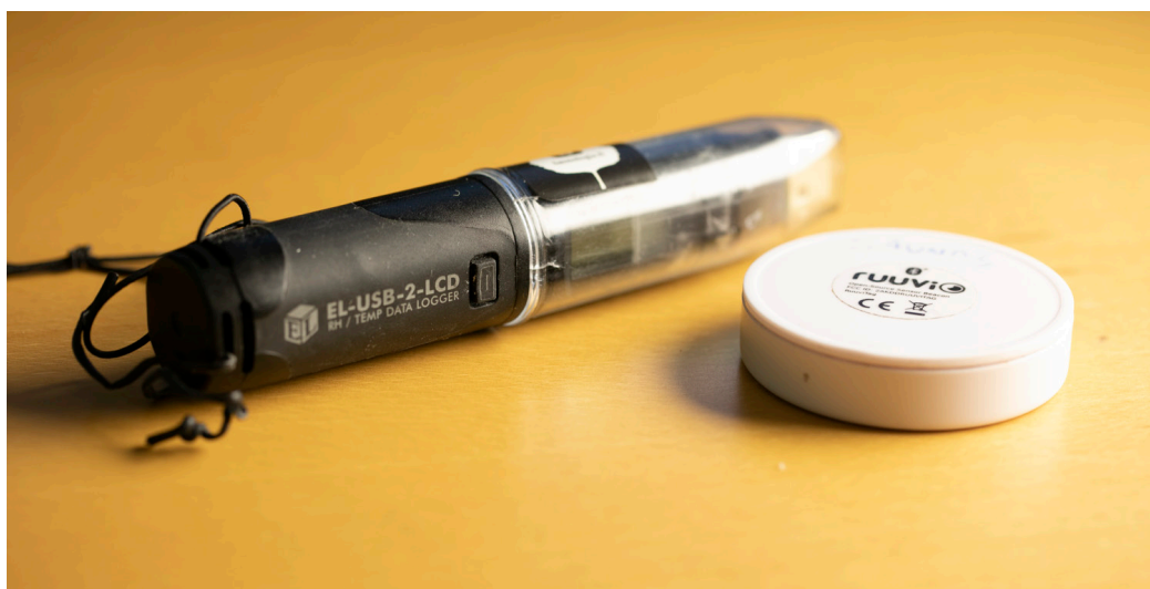
Figure 53. In my sauna studies, I commonly rely on digital thermometers with either built-in data logger or external data logging application. This is for convenience of later observation, traditional thermometers are also quite accurate. On the left a logger by Lascar Electronics, on the right a modified Bluetooth sensor by Ruuvi.
