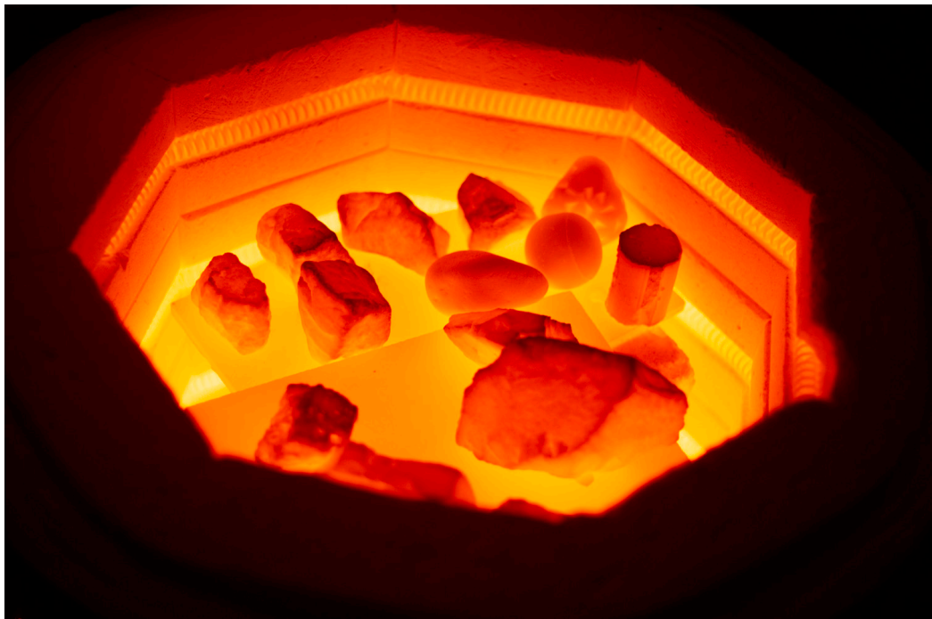
Figure 84. In an easy durability trial, I exposed a selection of stones to up to 750°C (1380°F) for a short period of time. This should be nothing for durable stones. Regardless of what the object is made of, they have deep red glow after some 600°C (1110°F) Celsius.
