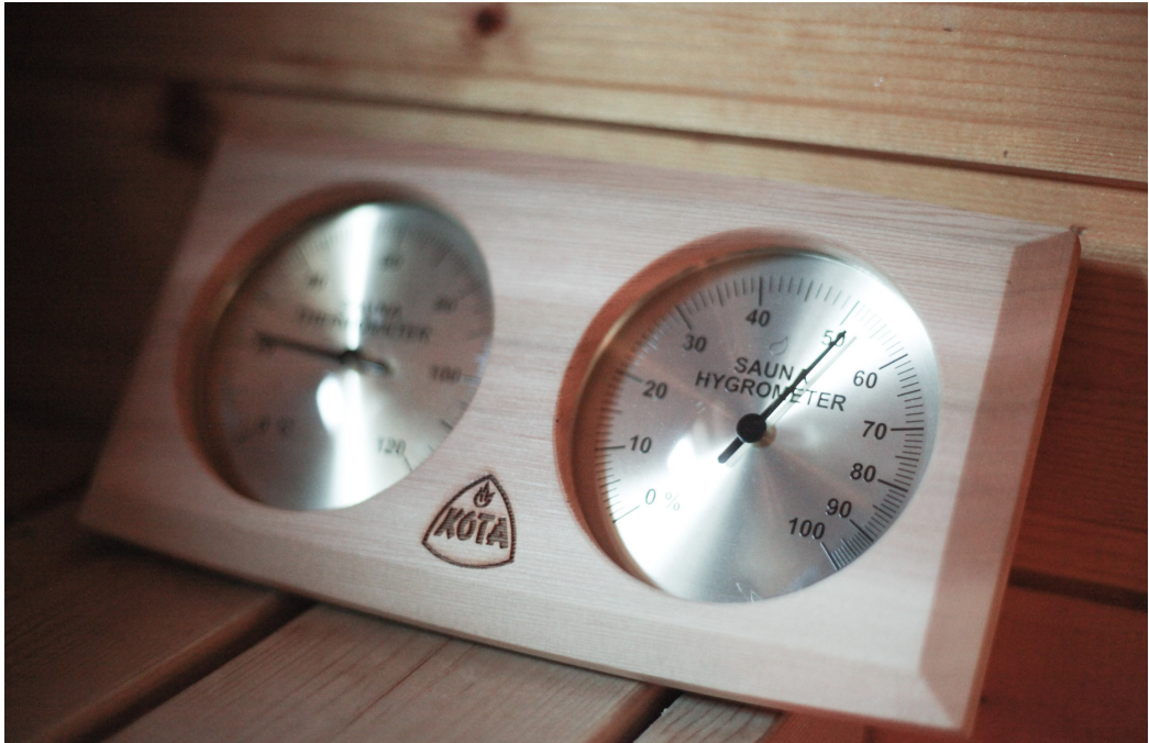
Figure 34. Sauna thermometer and hygrometer tell a story about the sauna climate. Finnish thermometers usually range up to 120°C (248°F).
