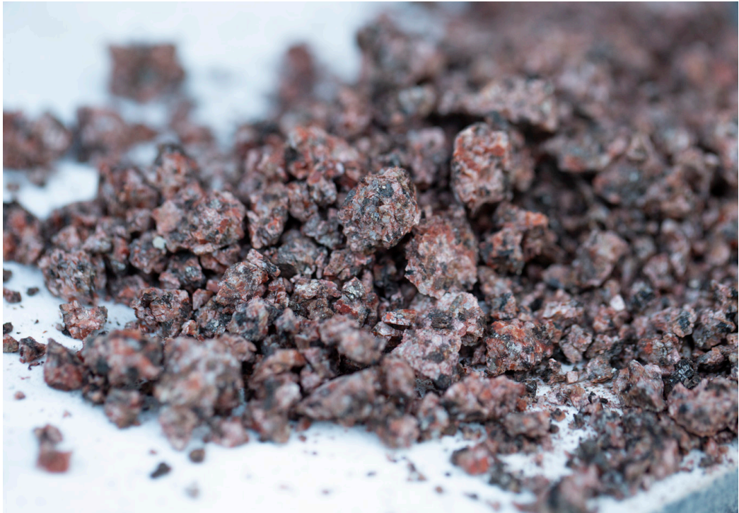
Figure 83. It does not get worse than this. A granite stone has totally collapsed under 500°C (930°F) heating. You don't want this to happen inside your heater.
