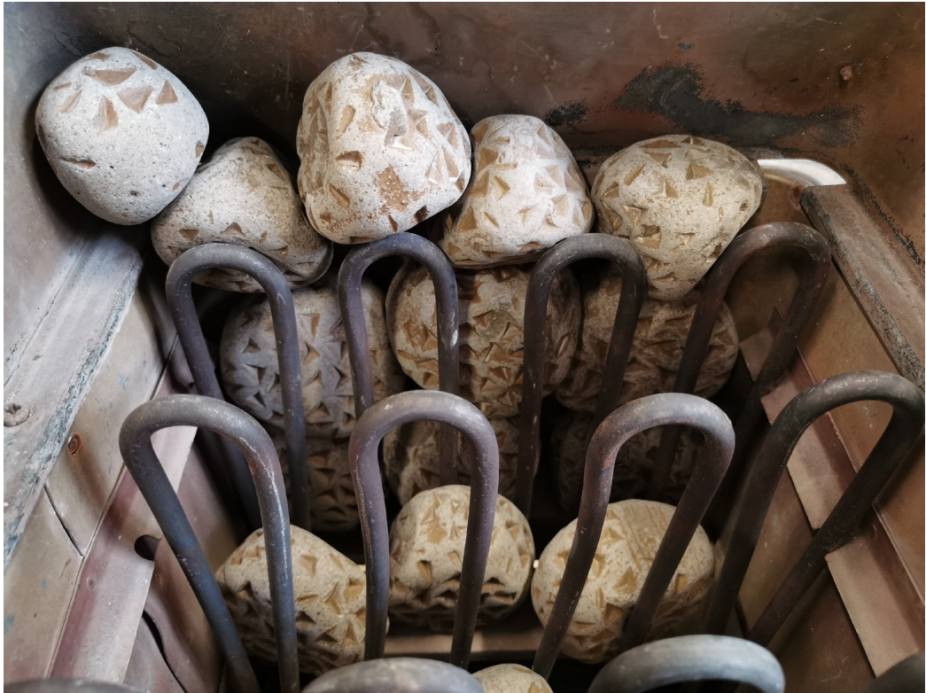
Figure 52. An old electric heater exposes still working key components: upward pointing heating elements and a few layers of ceramic “stones” which leave air space enough for a good convective flow through the heater.
