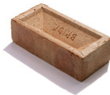
Frogged brick A commonly found brick with indentations on the top and bottom when laid in the stretcher position. The term 'frog' usually refers to the indentation, though it can also refer to the block which makes the indentation in the moulding process. Frogged bricks are lighter than solid bricks and the frogging also provides a great surface area for the mortar to adhere to when laid in courses.
