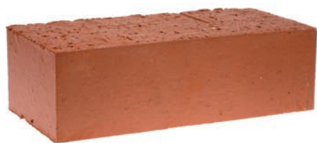
Solid brick A small cuboid of fired clay.
