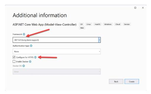
Figure 30-3. Configuring the ASP.NET Core MVC based Web Application template
