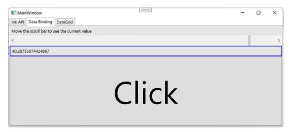
Figure 26-22. Binding the ScrollBar value to a Label and a Button
