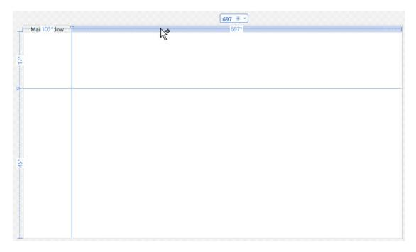
Figure 26-10. The Grid control can be visually cut into cells using the IDE's designer
