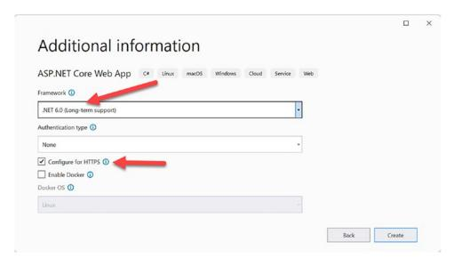
Figure 30-4. Configuring the ASP.NET Core Razor page MVC Web Application template
