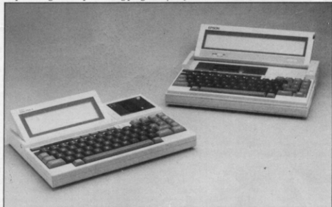
The Talbot Dialect 4 appears at first sight to be a cut down version of the Epson PX-8 (right). Obviously the display on the Talbot is half the size, so some software will not work. Programs stored on micro cassette will load however, which allows you to transfer text from one machine to the other. Unfortunately, the utility ROMs are not compatible, so you can't use Intext on a PX-8. But, Basic programs can be swapped between the two machines without too many problems.
