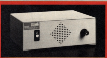
TALK SHOW — It may not be much to look at, but the Cambridge Microcomputer Centre's Namal SC10 prefers to let technology speak for itself. The unit is a 'type and talk' dedicated speech computer — with a Z80, a Votrax speech chip, and 10K of assorted memory it converts typed text into speech. You can connect it to 'any computer with RS232 serial link or Centronics parallel link,' CMC says, and it promises a number of refinements that aren't too common in this type of device — pronunciation of various symbols, adjustable speed, four inflexion levels, variable delay times between phrases and a choice of modes. CMC is on 0223-355404. The SC10 costs £149 plus VAT.
