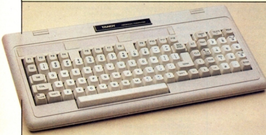
The keyboard doesn't wholly toe the IBMible line: the function keys are across the top, rather than down the side.
