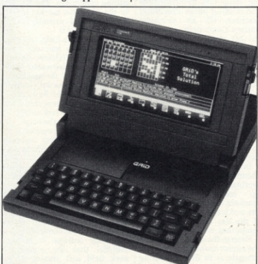
COMPASS ROSE — Grid Systems, maker of stylish and sturdy portables that find homes in Defence establishments and Space Shuttle programmes, has released two new versions of its Compass, along with software for more down to earth users. The new systems have 25 line electroluminescent screens with 128 characters a line, and they will set you back anything up to £7,950. The software packages have familiar names — GridMaster, GridPaint and GridTask. GridPaint costs £350 and the other two £250 each. The machine and software are distributed in the UK by Thame Systems.
