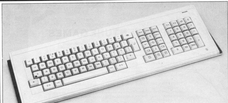
The keyboard layout has a Super shift key and two control keys, guarding the space bar.
