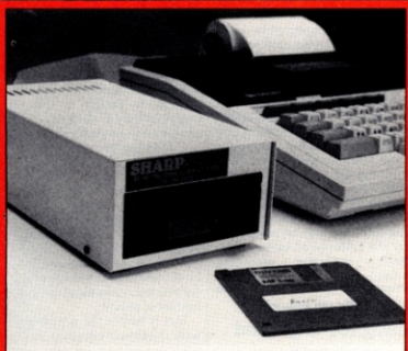
SHARP SPINDLE — A 3.5-in disk drive from Sharpsoft (01-739 8559) should give your MZ 700's memory a jolt. At £287 the MFD 700 has an inbuilt disk controller which means you don't need any further boxes. With 180K of memory, the Disk Basic that comes with the drive is compatible with Sharp's Basic and leaves 31K of user RAM. With the disk drive hooked up to your MZ 700 you will be able to use an extra 21 commands — a nice touch on a programmer's system.
