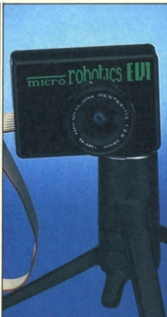
The camera includes an eight way cable for connecting to the computer and a small tripod.
