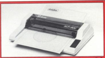
SMOOTH MOVER — Previously, biro printer plotters moved the paper vertically and were only capable of using half A4 width paper. Datafax has solved the width problem by using a mechanism similar to the HAL Sweet P plotters. The SCP-800 4 Colour Plotter Printer moves the paper via a pinch wheel on each edge. The same pin mechanism as on other biro plotters (Tandy, Atari, Oric etc) is used, ie the rotating four pin holder and solenoid to hammer them into the paper.
