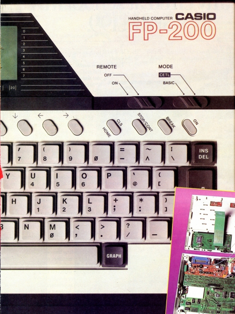
What's Inside the Casio FP-200 — 8K of RAM, expandable to 32K, plus the Casio C85 Basic
