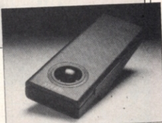
Heat-seeking mouse — infra-red connection and twin functions in a device that can be a mouse from one angle and a trackerball from another.
