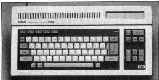
The Yamaha keyboard has a nice feel — the layout is standardised by the MSX conventions. The beloved diamond arrangement of the cursor keys has been substituted with a square.
