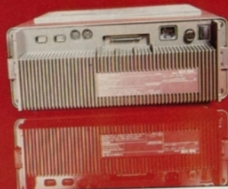
The Commodore SX64 — portable version of the best-selling 64 with built-in 5in colour monitor and disk drive. Expansion slots are on the underside with cartridge slot on top.
