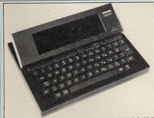
HANDY PORTABLE — Olivetti has joined the ranks of Tandy and NEC with its own portable called the M10. About the size of an A4 sheet of paper the M10 has a pop-up, 40 × 8 display screen, query keyboard and 32K ROM which contains the Basic interpreter, text editor, address book and diary. Two versions of the machine will be available — an 8K model at £499 or 24K at £699. You can get your first glimpse of the M10 plus its add-ons at Compec '83, Olympia London.
