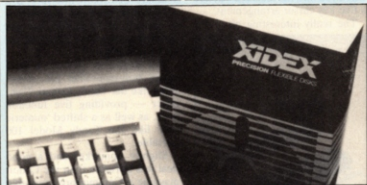
MAGNETIC FLOPPIES — Another addition to the mass of floppy disks on the market is Xidex's new line of 5 1/4 in and 8 in Precision flexible disks. With 96 tracks per inch the disks are made of the latest magnetic materials, the company says. To reduce head-to-disk interference problems due to shifting of the disk in the drive, Xidex has improved the tolerance on the inside diameter of the disk's centre hole by fifty per cent. Contact BFI, 01-941 4066.
