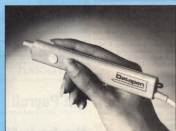
PEN PORTRAIT —For BBC, Dragon and Ic users who like dabbling on the screen, here's a new style of light pen. Datapen comes with a range of software at £25. It has an LED readout and a positioning switch. In addition to user routines and example programs, the company (also called Datapen) is providing a freehand drawing program. It is currently awaiting a technical drawing program that allow symbols to be created in a library and then combined on the screen. Contact Datapen on Overton (0256) 770488.
