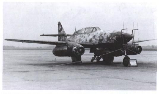
The Me-262 would not look out of place on a present-day airfield. It was soon fitted with accessories – external fuel-tanks to increase the range, and radar equipment, with the aerials mounted on the nose. (Cody Images)
