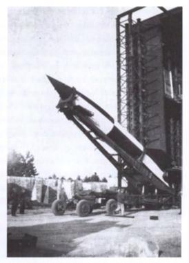
Operation Backfire was a British venture designed to evaluate the V-2 rocket system. Following the fall of Nazi Germany, flight tests were undertaken at a gun testing range at Cuxhaven, part of the British zone of occupation. (SSPL/Getty Images)
