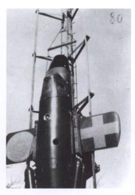
Engineers developed the Bachem Ba-349 Natter (Viper), a rocket-propelled interceptor. It was launched vertically from a rig that was difficult to detect from the air. (Cody Images)
