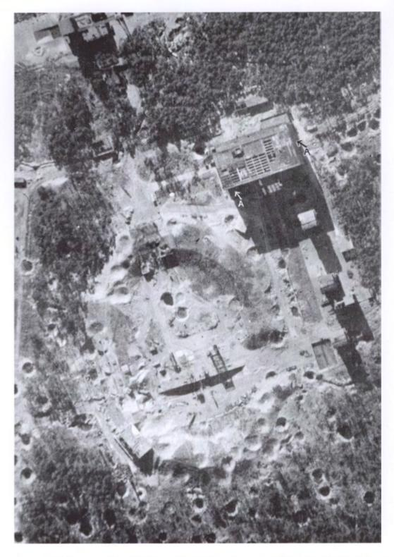
An annotated enlargement of a vertical photographic reconnaissance aerial picture taken over Test Stand VII in the German Army Research Centre, Peenemünde, after the heavy bombing attacks by aircraft of Bomber Command in 1943. As a result of the attacks, Peenemünde became inoperable and V-2 development was moved to Blizna in Poland. (IWM C 4783)
