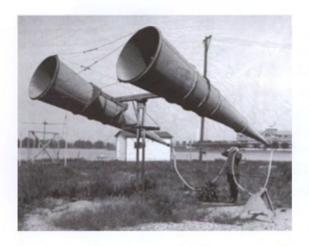
Experiments with sound receivers developed after World War I. As electronic amplifiers were yet to be perfected, acoustic horns were used instead. These detectors were used to detect distant aircraft. (Library of Congress)
