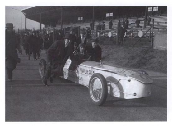
Max Valier pictured here in his rocket car, designed in 1929. He experimented with rocket vehicles and died when an alcohol-fuelled rocket car exploded in 1930. (Bundesarchiv Bild 1020-01350)
