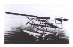
The Ar-231 was designed as a lightweight seaplane for carrying aboard a U-boat, allowing it to attack Allied shipping with minimal flying time. It was never used in the war due to its instability and lack of power. (Cody Images)
