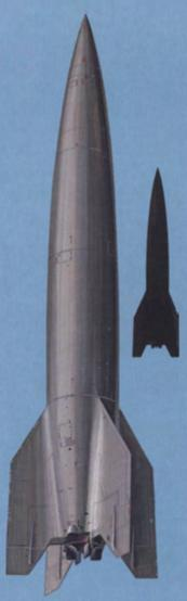
The V-2 was an intercontinental ballistic missile weighing 28,000lb (12,700kg). It stood 46ft (14m) tall and was 5ft 5in (1.65m) in diameter. With an operational velocity of 3,580mph (5,760km/h) – more than twice the speed of sound – it could travel over a distance of 220 miles (320km) and deliver 2,200lb (980kg) of Amatol high explosive. The design was re-used by the US as the the Redstone rocket after the war. (John Batchelor)
