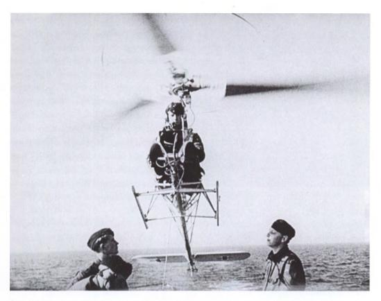
Gyrogliders were used for observation in World War II and the Focke-Achgelis Fa-330 could be easily dismantled and stored in a small container on a U-boat. It was used for spotting ships at distance while being towed behind the submarine. The submarine could rapidly submerge, usually (but not always) with the kite pilot safely back on board. (EN Archive)
