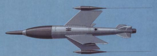
Guided by wire that unspooled as it flew, the X-4 8-344 air-to-air missile was designed by Max Kramer at Ruhrstahl in 1943. It was powered by a BMW 109-548 rocket engine and carried a warhead containing 44lb (20kg) of high explosive with a destructive range of 25ft (7.6m). This missile had a top speed of 716mph (1,152km/h) and the control cable was 3.4 miles (5.5km) long. Although roughly 1,000 were built, the Kramer missile was never used in the war. (John Batchelor)
