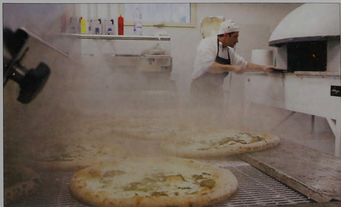
A fine mist of liquid nitrogen gently freezes pizzas as they traverse down a conveyor belt over the course of 10 minutes.
