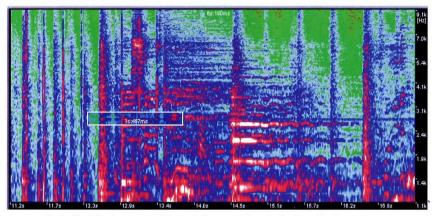
The feedback has been removed. Intepolation occurred vertically, from other frequency elements played at the same time.
