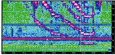
Complex filtering in Renovator. Hum at 50 and 100 Hz has been selected
