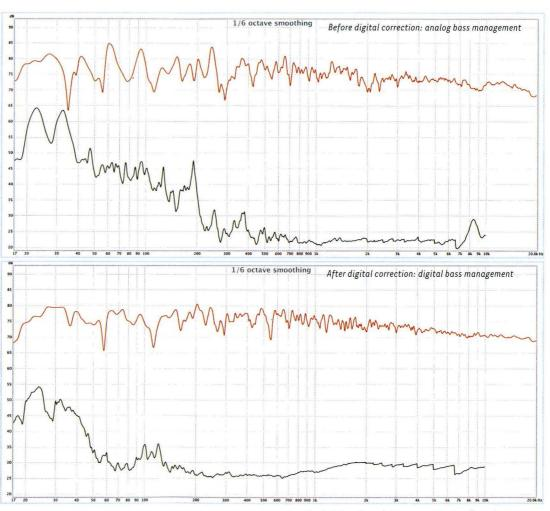
Left front channel frequency response, 1/6 octave smoothing, 500 ms fixed window (brown). Harmonic distortion (black).
