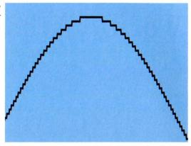
Pictured above is a portion of a sine wave that has been quantized without dither. Since there is no resolution below the level of each quantization step, the result is a stepped, distorted waveform. Low-level information is completely lost. To prevent this kind of distortion, we use dither, which is a process that mathematically removes the highly undesirable distortions entirely, and replaces them with a fixed noise level.
