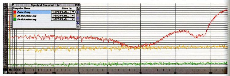
POW-R type 3 dither at 44.1 kHz/16-bit (red trace), compared with 20-bit flat dither (orange) and 24-bit flat dither (green).
