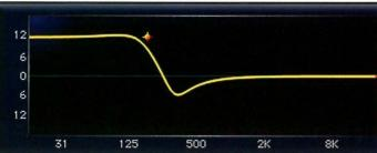
Top: Gerzon resonant shelf with a low Q. The dip just past the shelving boost frequency is characteristic of the Gerzon resonant shelf. Bottom: The same with a high Q.
