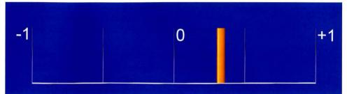
Correlation Meter reading almost 3/4 of the way towards the right, which indicates only moderate stereo separation and likely a fairly narrow stereo image.
