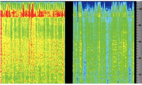
Above left is a spectragram of the distortion created when converting a smashed and clipped CD to mp3. At right, the distortion when converting an "ordinary" loud CD which was brickwall limited and not clipped.
