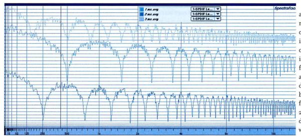
Severe Comb Filtering
