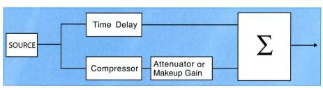
The Parallel Compression technique employs a matched time delay in the "dry" signal path to avoid phase shift or comb filtering.  $\Sigma$  is the symbol for "sum." This yields very transparent-sounding upward compression.
