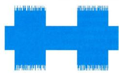
With attack/release too fast, a compressor can produce severe distortion.
