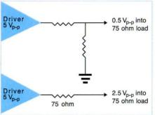
Voltage level improvement for S/PDIF transmitter
