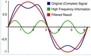
Shown in blue is a complex wave. When the high frequency information (green) is filtered out, the result is a signal (red) that is higher in amplitude than the original! Image created by B.J. Buchalter.
