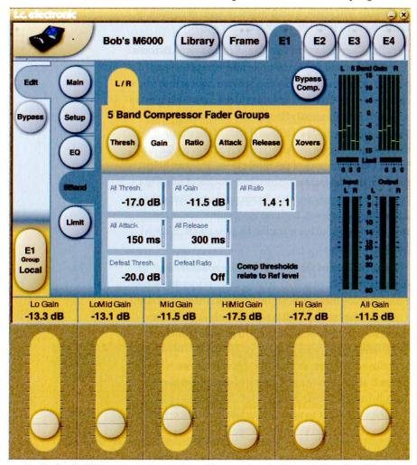
Tonalization: The TC MD4 performing "warming" parallel compression using higher gains in the low mid band.
