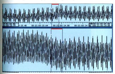
Figure B After manual declicking, the right channel thunk has been removed.
