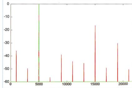
Figure D Spectrum of original sine wave in green, clipped spectrum in red
