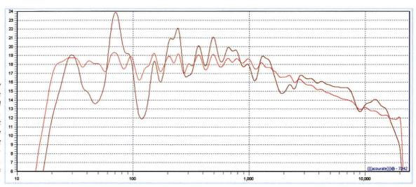
Left front channel frequency response, psychoacoustic measurement, uncorrected (brown), corrected (red). Psychoacoustic measurement uses a continusly-variable FFT window, from very long at low frequencies, to nearanechoic at high frequencies, the way that the ear responds to sound.
