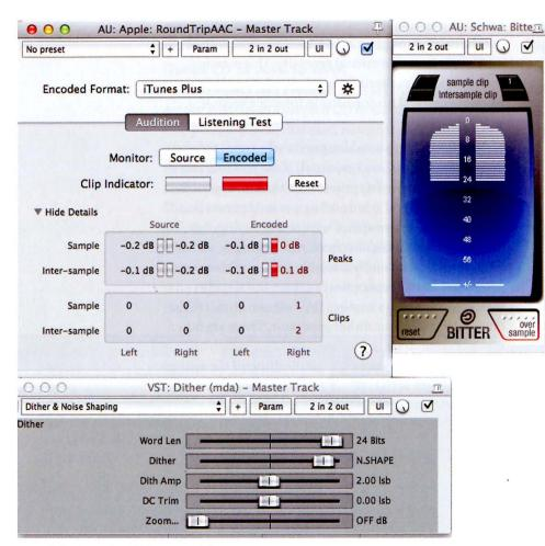
Dither the result to 24 bits so it sounds best when listening on a DAC, or for conversion to a 24-bit wav. Engineers might want to reduce the amplitude to prevent clipping, as shown both in Apple's plug-in and in Bitter. We don't hear the 24-bit dither noise directly — its amplitude is too low, but we do notice the slight improvement in sound due to the reduction of distortion, which would have been above the noise floor of the DAC.
