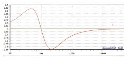
Phase graph of a 100 Hz parametric boost. In green, linear phase, in red, minimum phase.
