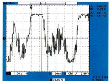
A severely-clipped waveform from a contemporary CD
