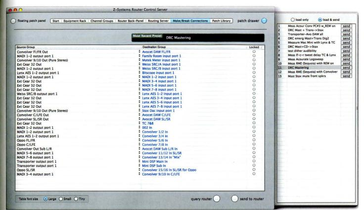
a digital mixer. A 16x16 router is sufficient for a small mastering studio, but a medium size studio processing stereo and a small amount of multichannel work would require a 32x32 router, and the largest studios need 128x128 or larger. Since AES/EBU carries 2 channels, a 128x128 router actually switches 256 channels in pairs. There are two basic types of digital routers:
