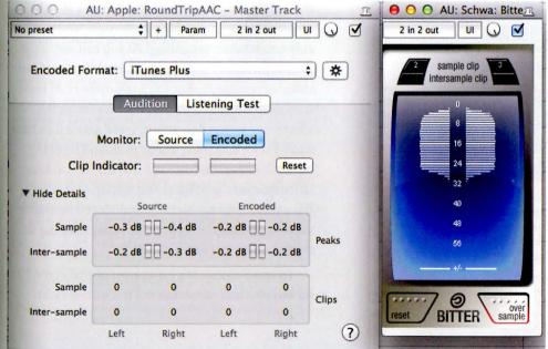
PCM fixed-point source file encoded to AAC, then decoded to PCM. Notice there are now 32 active bits.
