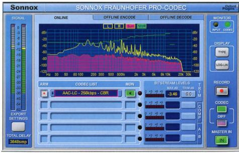
Fraunhofer Pro-Codec by Sonnox. Demonstrate the effects of coding with any chosen codec or bitrate. On Windows it is not the exact AAC codec used by OSX, but it is close. Also can convert any file(s) between coded and PCM for later comparison in a DAW without the plug-in.
