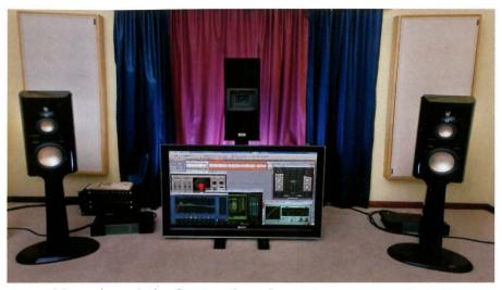
Custom video monitor mount places it on the floor, avoiding interference with the sound produced by the main speakers.
