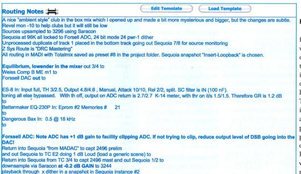
Mastering log containing routing and analog processor settings. Digital processor settings are loaded from a Sysex dump.
