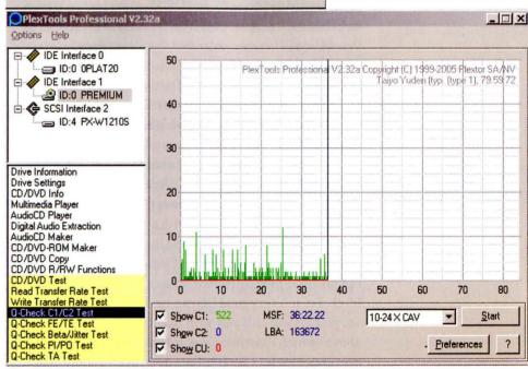
There is also the issue of *error concealment*, which is the last defense mechanism in digital playback. If there is an uncorrectable error of fairly short duration, instead of muting, the playback machine interpolates between the audio level before and after the error. Short bursts of error concealment can be virtually inaudible or smooth the sound pleasantly, but professionals never use a master medium that is so degraded. So we verify
