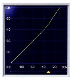
An upward expander with .75:1 ratio, expressed in decimal (1:1.33 expressed as a fraction). Threshold is -32 dBFS, and without attenuation, the output will overload if input exceeds approximately -10 dBFS.
