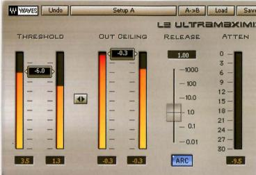
The Power of Floating-Point Processing: The first processor in the chain shows an "overload" (+3.5/+1.3). This level is cleanly passed via floating point to the Waves L2, which shows the identical "over" input levels. Yet it can still peak limit effectively and output a signal that is not clipped.
