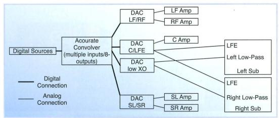
Digitally-corrected 5.1 monitor system with a 5x3 digital 2-way crossover
