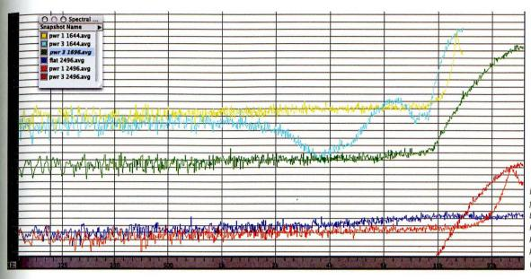
Dithers at different sample rates, from highest to lowest level. At 16-bit/44.1 kHz: POW-R 1 (yellow) and POW-R 3 (turquoise). At 16-bit/96 kHz: POW-R 3 (green). At 24-bit/96 kHz: flat dither (blue), POW-R 1 (orange) and POW-R 3 (red).
