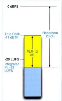
The same program loudness-normalized for EBU broadcast, with target of -23 LUFS. Note that the sound quality has been maintained, since the PLR remains the same. Headroom has increased. Since the 24-bit noise level is already inaudible, there is no perceptible signal-to-noise ratio difference.
