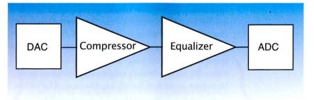
D/A/D Processing Chain. The choice of whether to place compressor or equalizer first depends on the intent. See text.
