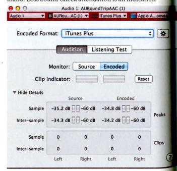
Apple's AU Round Trip AAC plug-in. It allows comparison between PCM source and AAC encode, and measures clips.
