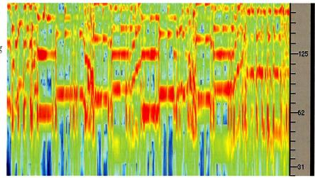
SpectraFoo<sup>™</sup> spectragram of the bass frequencies of several measures from a rock piece. Read it like an orchestra score, time runs from left to right. Red represents the highest levels. The bass runs in the 62–125 Hz fundamental range are paralleled by second and third harmonics.
