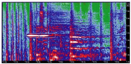
Acoustical feedback has been identified by drawing a box around the offending sound.
