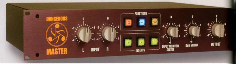
Dangerous Master transfer console. Insert and level functionality with MS width control and valuable source level offset for level-matching mix versus master.
