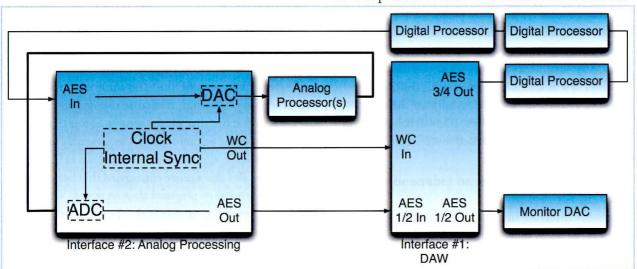
Mastering system block diagram.
