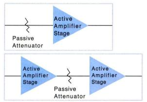
In the top device, signal enters a passive attenuator and exits through an active amplifier stage. This circuit effectively has infinite input headroom. The bottom device's input headroom is determined by the headroom of the input amplifier.
