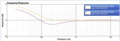
Pultec response curve obtained by simultaneously applying bass boost and bass cut.
