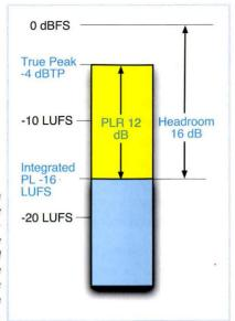
Example music program: Program loudness in blue at -16 LUFS. True peak level at -4 dBTP. The difference between these two is the PLR, 12 dB. Headroom is defined as the difference between the program loudness and the peak capability of the medium, which in this case is 16 dB.
