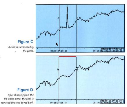
In Figure C (above) a severe click is marked manually by the gates, and in Figure D it has been removed. Note that Sonic Solutions' automatic vertical gain conveniently amplifies the display to the highest amplitude in the view.
