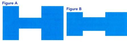
Figure A: a simple tone burst from high to low level and back. Figure B: the same tone burst passed through a compressor with very fast attack, high ratio, and fast release time.
