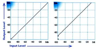
Three transfer curves. (From left to right). Amplifiers with Unity-Gain, 10 dB gain, and 10 dB loss (attenuation).
