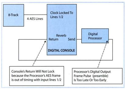
AES to AES framing error can cause locking problems
