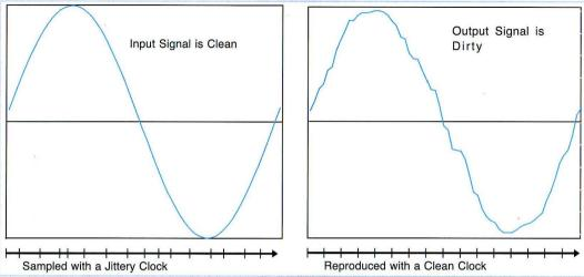
Jitter during A/D conversion creates permanent distortion
