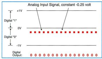
Graph of a hypothetical ADC whose LSB threshold is 0 volt. Each sampled analog input is represented by an orange square; in this example, the analog source is held at a continuous -0.25 volt. Note that any input between -1 volt and 0 volt will be lost, because it is below the threshold of the LSB, producing a string of zeros. Because it is below threshold, this signal at -0.25 volts will not be detected, and it will be truncated to a value of 0.
