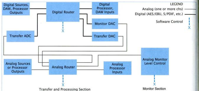
The ideal mastering studio (block diagram) has all these elements. Routers, manual switches or patchbays interconnect the gear, either manually or under software control.
