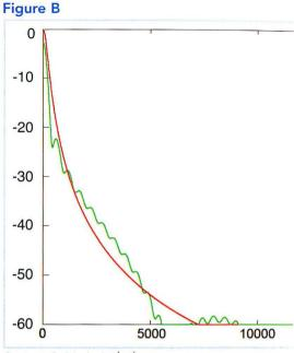
Spectrum of original pulse (red), spectrum of clipped pulse (green).
