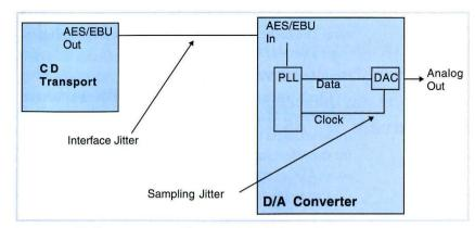
has a good PLL, no external box can help. Many of these clock generators hurt the sound if you pick the wrong unit and/or it is not compatible with the PLL in your converter.
