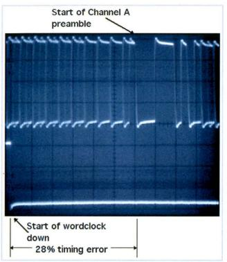
This oscilloscope photo compares the timing of the start of the Channel A AES preamble against the start of wordclock at the output of a digital processor. This timing offset of 28% of the length of the AES frame is 3 points greater than the permissible tolerance in standard AES11 and would cause locking trouble to intolerant consoles or DAWs or other receivers.
