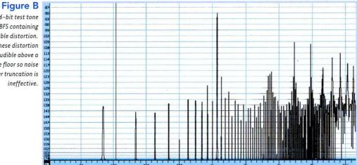
than -130 dBFS in a 16-bit dithered system, although -130 is too low to be heard because it is masked by the dither noise (Figure A above). Figure B illustrates the severe distortion that would occur if this signal were not dithered. The perceived (audible) dynamic range of a dithered system is greater than it can code, because human beings are able to hear signals in the presence of noise of greater energy than the signal. We can hear
