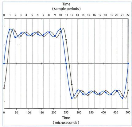
Sample rate does not limit the timing resolution of digital audio as illustrated here where two waves are offset by less than half a sample period. Image courtesy of Dick Pierce ©2007.
