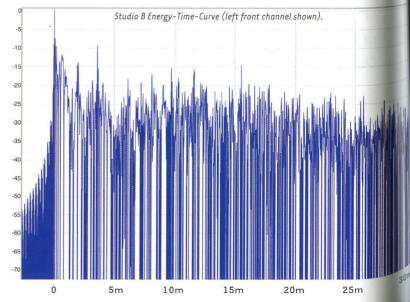
Reflections are serious business. Poor time-domain response means poor frequency response. The sound of Darth Vader's voice in Star Wars is a comb filter created by mixing in a delay at 10 ms with the dry sound.<sup>1</sup>
