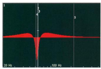
"One-note bass" resonance fixed by a combination of a shelving boost (which was useful to help the rest of the notes that were weak) and a narrow band dip at the resonance frequency.
