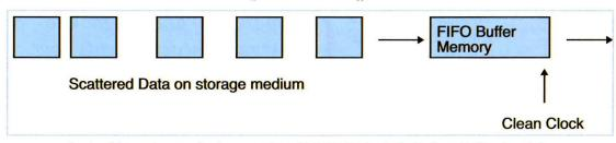
Spacing of data on storage medium has no meaning as it is first buffered and output to the world with a clean clock.
