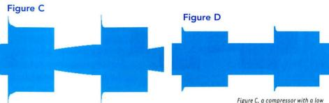
ratio, slow attack time, and slow release time. Figure D, higher ratio, faster attack and very fast release.
