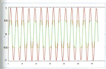
Figure C 5 kHz sine wave, unclipped (red), clipped (green).
