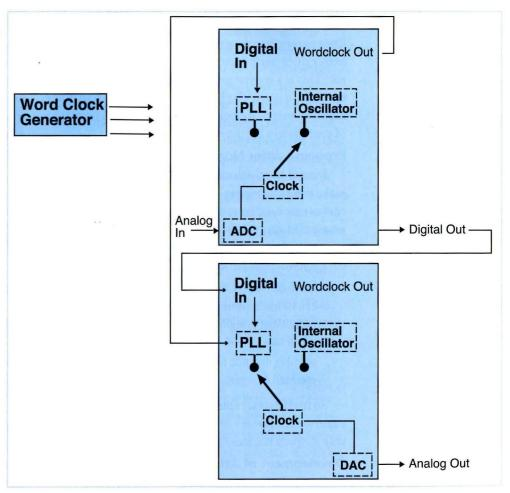
Jitter is more difficult to control when ADC and DAC are in separate boxes
