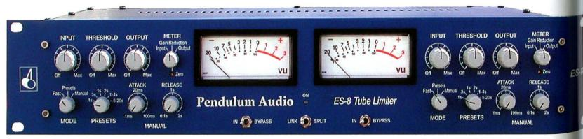
Pendulum Audio ES-8 variable mu (remote cutoff triode) tube compressor with transformer coupled input and transformerless solid-state balanced line output. It's far more transparent than the Fairchild but can be warm, punchy or creamy when you need it, very versatile. See discussion in Chapter 6.
