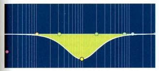
Simple midrange dip. Notice that the high and low frequencies are flat.
