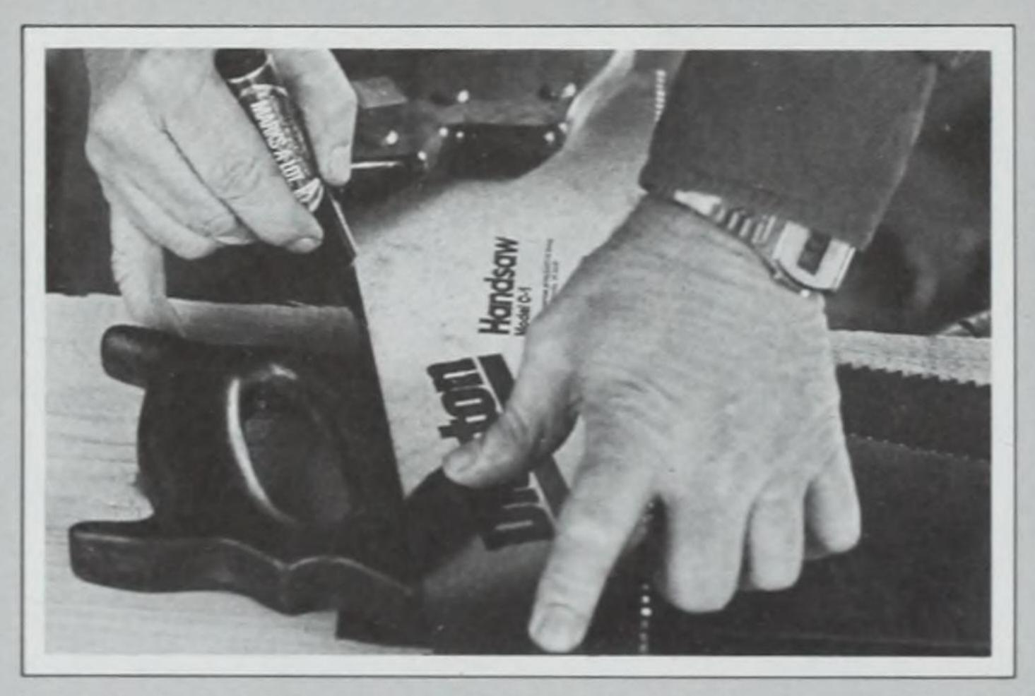
3—I used an old saw I was trying to match as a pattern for the new saw and marked the old Disston for recutting. Note the angle of the slot that must be cut in the new handle. The aft end of the old saw is marked for cutting so that it will match.
