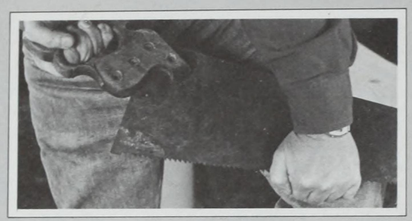
1—The recycling work on this old Disston saw starts with pulling off the old handle.
