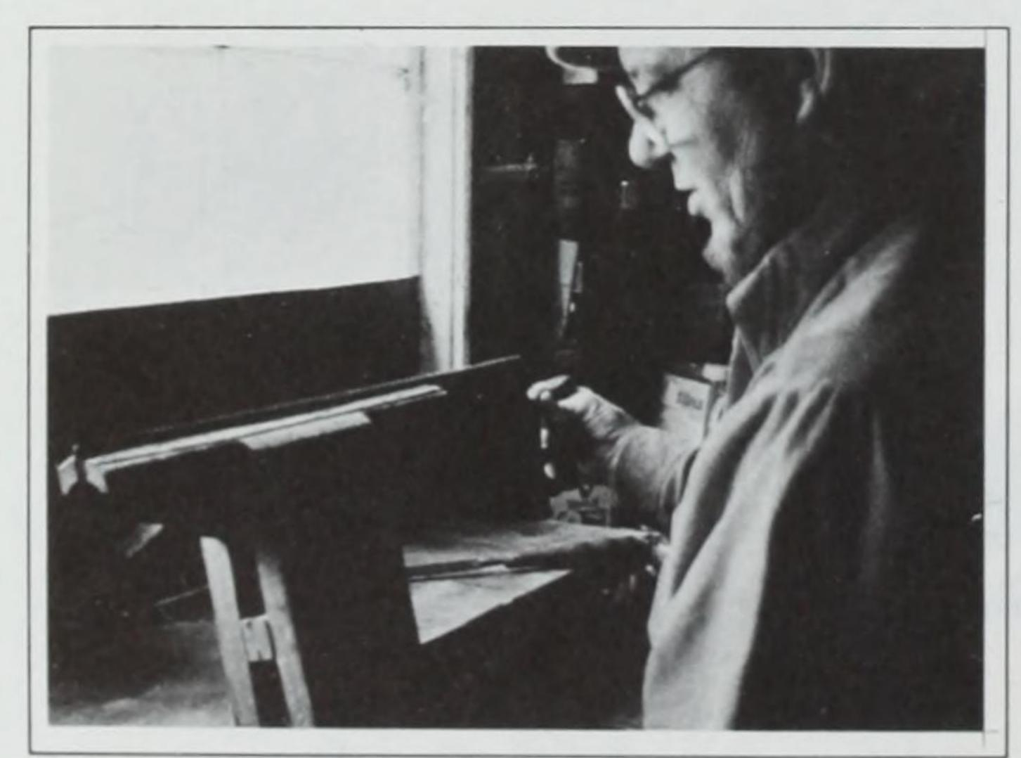
The saw can be put in the vise with its handle in either direction. Natural light is essential, but the lower windowpanes are blocked off so that...
