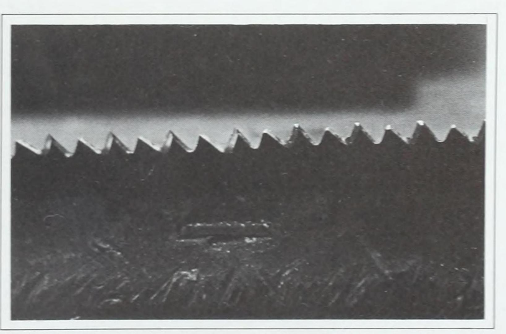
Notice the sharp teeth on the left side of this saw (about 10 of them) and the dull teeth on the right. The dull teeth shine because their points have just been jointed, but they haven't been filed yet.
